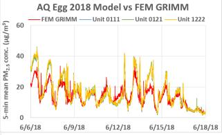
Coefficient of Determination (R<sup>2</sup>) quantifies how the three sensors followed the PM<sub>2.5</sub> concentration change by FEM.
