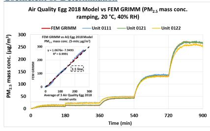
The Air Quality Egg 2018 Model sensors showed very strong correlations with the corresponding FEM PM<sub>2.5</sub> data ( $R^2 > 0.99$ ) at 20 °C and 40% RH.
