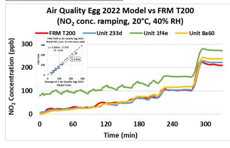
The Air Quality Egg 2022 Model sensors showed very strong correlations with the corresponding FRM T200 NO<sub>2</sub> data (R<sup>2</sup> = 0.99) at 20 °C and 40% RH.
