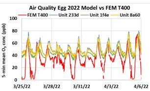
Coefficient of Determination (R<sup>2</sup>) quantifies how the three sensors followed the O<sub>3</sub> concentration change by the reference instruments.
