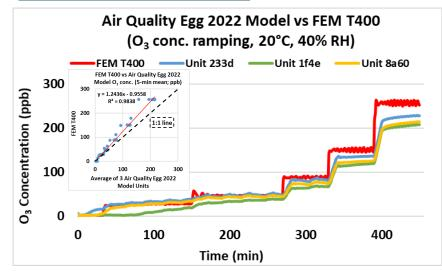
The Air Quality Egg 2022 Model sensors showed very strong correlations with the corresponding FEM T400 O<sub>3</sub> data (R<sup>2</sup> ~0.98) at 20 °C and 40% RH.
