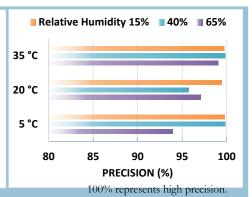
Sensor's ability of generating precise measurements of PM concentration at low, medium, and high pollutant levels were evaluated under 9 combinations of T and RH, including extreme weather conditions like cold and humid (5 °C and 65%), hot and humid (35 °C and 65%), cold and dry (5 °C and 15%), and hot and dry (35 °C and 15%).
