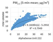
Coefficient of Determination (R<sup>2</sup>) quantifies how the three sensors followed the PM concentration change by FEM.
