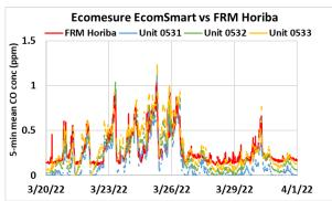
Coefficient of Determination (R<sup>2</sup>) quantifies how the three sensors followed the CO concentration change by the reference instruments.
