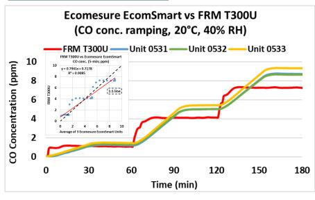
The Ecomesure EcomSmart sensors showed very strong correlations with the corresponding FRM T300U CO data ( $R^2 \sim 0.91$ ) at 20°C and 40% RH.
