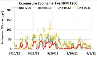
Coefficient of Determination (R<sup>2</sup>) quantifies how the three sensors followed the NO<sub>2</sub> concentration change by the reference instruments.
