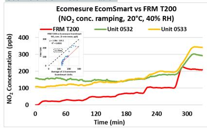
The Ecomesure EcomSmart sensors showed strong correlations with the corresponding FRM T200 NO<sub>2</sub> data ( $R^2 \sim 0.89$ ) at 20°C and 40% RH.
