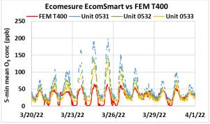
Coefficient of Determination ( $R^2$ ) quantifies how the three sensors followed the  $O_3$  concentration change by the reference instruments.
