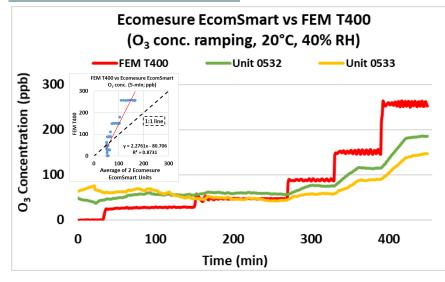
The Ecomesure EcomSmart sensors showed strong correlations with the corresponding FEM T400  $O_3$  data ( $R^2 \sim 0.87$ ) at 20°C and 40% RH.
