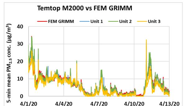
Coefficient of Determination ( $R^2$ ) quantifies how the three sensors followed the PM<sub>2.5</sub> concentration change by the reference instruments.
