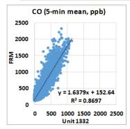
Coefficient of Determination (R<sup>2</sup>) quantifies how the three sensors followed the CO concentration change by FRM.
