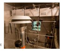
The sensor's readings at each ramping steady state are compared to the reference instrument.
