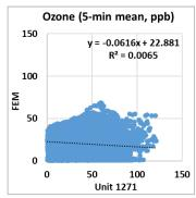
Coefficient of Determination ( $\mathbb{R}^2$ ) quantifies how the three sensors followed the O<sub>3</sub> concentration change by FEM.
