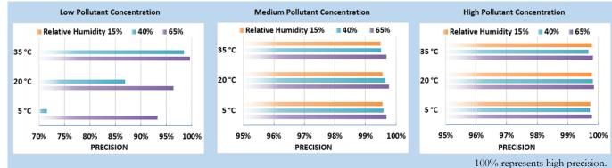
Sensor's ability of generating precise measurements of  $O_3$  concentration at low, medium, and high pollutant levels were evaluated under 9 combinations of T and RH, including extreme weather conditions like cold and humid (5 °C and 65%), hot and humid (35 °C and 65%), cold and dry (5 °C and 15%), and hot and dry (35 °C and 15%).
