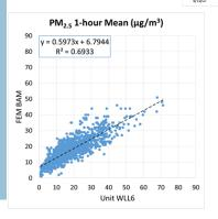
Coefficient of Determination (R<sup>2</sup>) quantifies how the three sensors followed the PM concentration change by the reference instruments.
