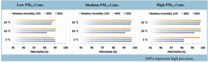
Sensor's ability at generating precise measurements of PM concentration at low, medium, and high pollutant levels were evaluated under 9 combinations of T and RH, including extreme weather conditions like cold and dry (5 °C and 15%), cold and humid (5 °C and 65%), hot and humid (35 °C and 65%), or hot and dry (35 °C and 15%).
