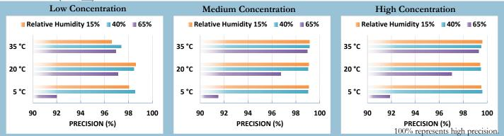
Sensor's ability to generate precise measurements of ozone concentration at low, medium, and high pollutant levels were evaluated under 9 combinations of T and RH, including extreme weather conditions like cold and dry (5 °C and 15%) cold and humid (5 °C and 65%), hot and humid (35 °C and 65%), or hot and dry (35 °C and 15%).
