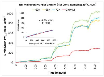
The three RTI MicroPEM sensors showed very strong correlations with the corresponding FEM PM<sub>2.5</sub> data ( $R^2 = 0.99$ ) at 20 °C and 40% RH from 0 - 250  $\mu$ g/m<sup>3</sup>.
