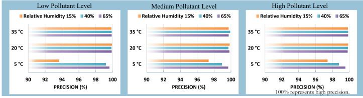
Sensor's ability of generating precise measurements of CO concentration at low, medium, and high pollutant levels were evaluated under 9 combinations of T and RH, including extreme weather conditions like cold and humid (5 °C and 65%), hot and humid (35 °C and 65%), cold and dry (5 °C and 15%), and hot and dry (35 °C and 15%).
