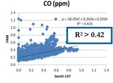
Coefficient of Determination (R<sup>2</sup>) quantifies how the three sensors followed the CO concentration change by FRM.
