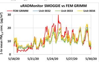
Coefficient of Determination  $(R^2)$  quantifies how the three sensors followed the PM<sub>2.5</sub> concentration change by the reference instruments.
