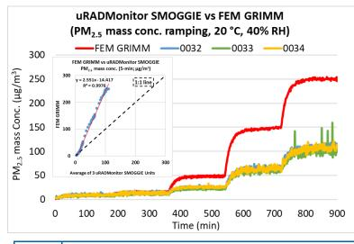
The uRADMonitor SMOGGIE sensors showed very strong correlations with the corresponding FEM PM<sub>2.5</sub> data ( $R^2 > 0.99$ ) at 20 °C/40% RH.. For conc. ramping experiments of PM<sub>1.0</sub>, please see the lab report.
