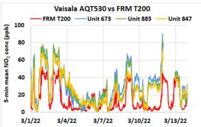
Coefficient of Determination (R<sup>2</sup>) quantifies how the three sensors followed the NO<sub>2</sub> concentration change by the reference instruments.
