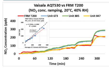
The Vaisala AQT530 sensors showed very strong correlations with the corresponding FRM T200 NO<sub>2</sub> data (R<sup>2</sup> > 0.96) at 20°C and 40% RH.
