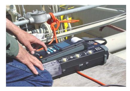
FOR THE PERIODIC MONITORING OF NITROGEN OXIDES, CARBON MONOXIDE, AND OXYGEN FROM COMBUSTION SOURCES SUBJECT TO RULES 1110.2, 1146, AND 1146.1
