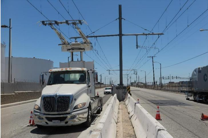
TransPower Catenary Truck on the OCS Track
