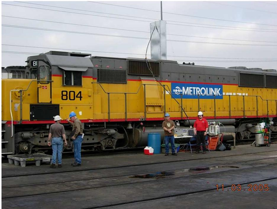
**Figure 2: Emission measurement system installation on Metrolink No. 800**
