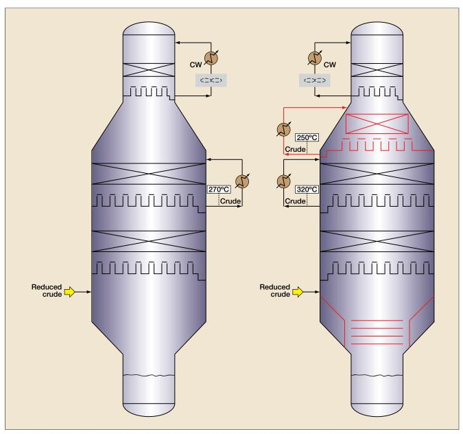
Figure 3 Vacuum tower MVGO pumparound
