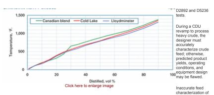
crude's heavy end has resulted in poor revamp yields and coked vacuum column wash beds.
