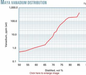
Table 3 shows how CFHT feed Fig. 3vanadium content can increase for a poorly designed CDU heavy crude revamp. High ATB entrainment into the atmospheric gas oil (AGO) and high entrainment and poor fractionation in the vacuum unit caused the high CFHT feed vanadium content.
