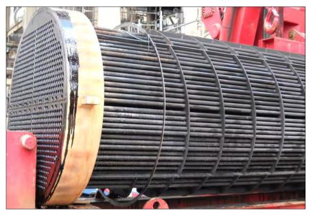
Figure 6 HelixChanger bundle after two years of operation in hot crude vs hot resid service
