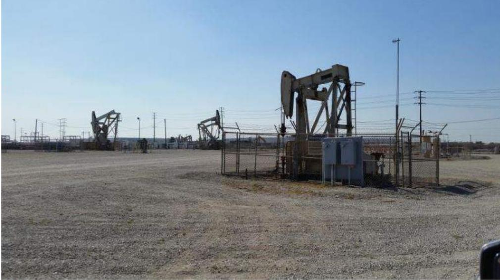
**Figure 2-14. Typical Well with Electric Pumpjack Located at 700 Block.**
