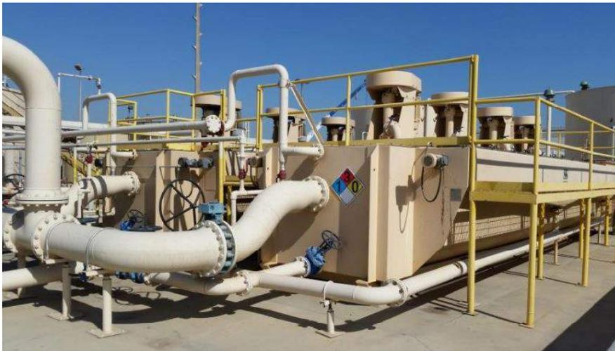
**Figure 2-8. WEMCO Separator at the 700 Block Main Facility.**
