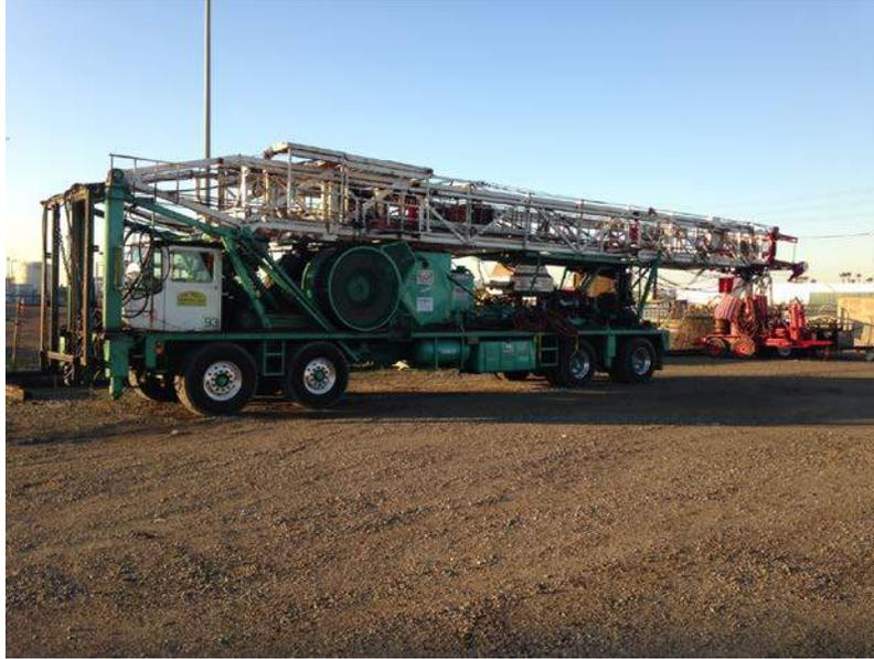
**Figure 2-16. Typical Well Workover Rig.**
