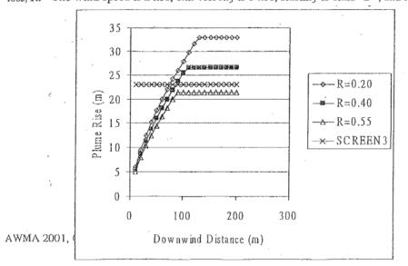
Figure 4. The predicted plume rise versus downwind distance for three values of radiant heat loss, R. The wind speed is 2 m/s, exit velocity is 6 m/s, stability is class "D", and load is 10%.
