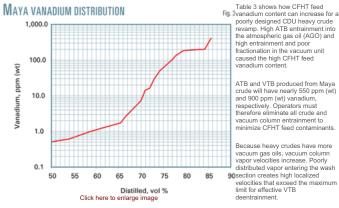
Some refiners have seen HVGO MCR and vanadium levels greater than 1 wt % and 10 ppm (wt), respectively, when processing 22° API gravity crudes. CFHT FEED STREAM VANADIUM Table 3
