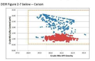
The DEIR did provide some information on crude oil at the two refineries. For example, the following graphics show sulfur % and API gravity spreads at the refineries (each point represents a different crude oil).
