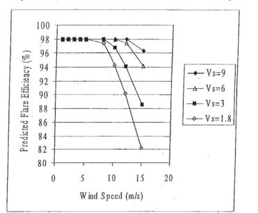
Figure 3. The predicted flare destruction efficiency (%) as a function of flare tip exit velocity ( $V_s$  in m/s) and wind speed (m/s). The radiant heat loss is 0.40 and the stability is class "D".
