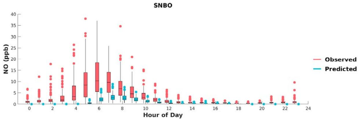
**FIGURE G-21: BOX PLOTS OF OBSERVED VS. PREDICTED HOURLY NO DURING MAY 1<sup>ST</sup> TO SEPTEMBER 30<sup>TH</sup>, 2018, AT SAN BERNARDINO. HORIZONTAL LINES INDICATE 25<sup>TH</sup>, 50<sup>TH</sup> (MEDIAN), AND 75<sup>TH</sup> PERCENTILES.**
