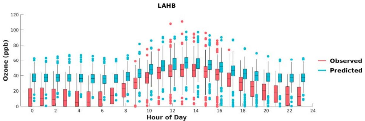
**FIGURE F-13: BOX PLOTS OF OBSERVED VS. PREDICTED HOURLY OZONE DURING MAY 1<sup>ST</sup> TO SEPTEMBER 30<sup>TH</sup>, 2018, AT LA HABRA. HORIZONTAL LINES INDICATE 25<sup>TH</sup>, 50<sup>TH</sup> (MEDIAN), AND 75<sup>TH</sup> PERCENTILES.**
