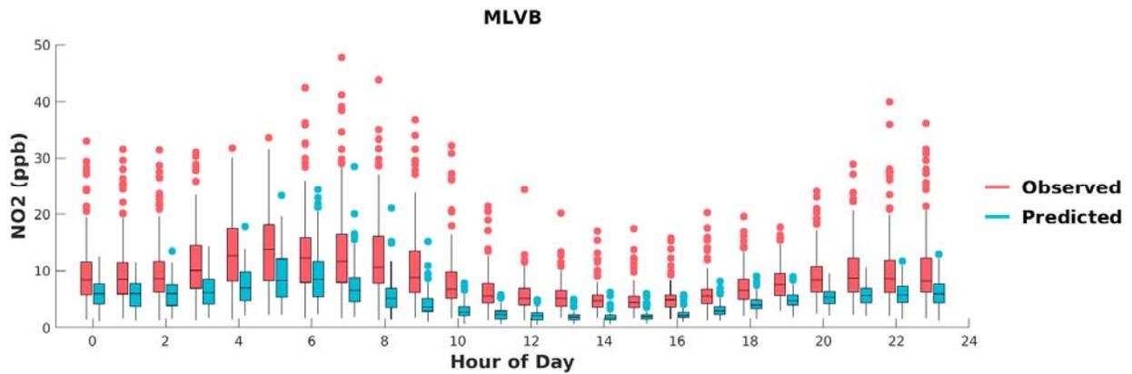
**FIGURE H-12: BOX PLOTS OF OBSERVED VS. PREDICTED HOURLY NO<sub>2</sub> DURING MAY 1<sup>ST</sup> TO SEPTEMBER 30<sup>TH</sup>, 2018, AT MIRA LOMA VAN BUREN. HORIZONTAL LINES INDICATE 25<sup>TH</sup>, 50<sup>TH</sup> (MEDIAN), AND 75<sup>TH</sup> PERCENTILES.**
