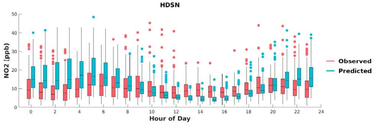
**FIGURE H-9: BOX PLOTS OF OBSERVED VS. PREDICTED HOURLY NO<sub>2</sub> DURING MAY 1<sup>ST</sup> TO SEPTEMBER 30<sup>TH</sup>, 2018, AT HUDSON. HORIZONTAL LINES INDICATE 25<sup>TH</sup>, 50<sup>TH</sup> (MEDIAN), AND 75<sup>TH</sup> PERCENTILES.**
