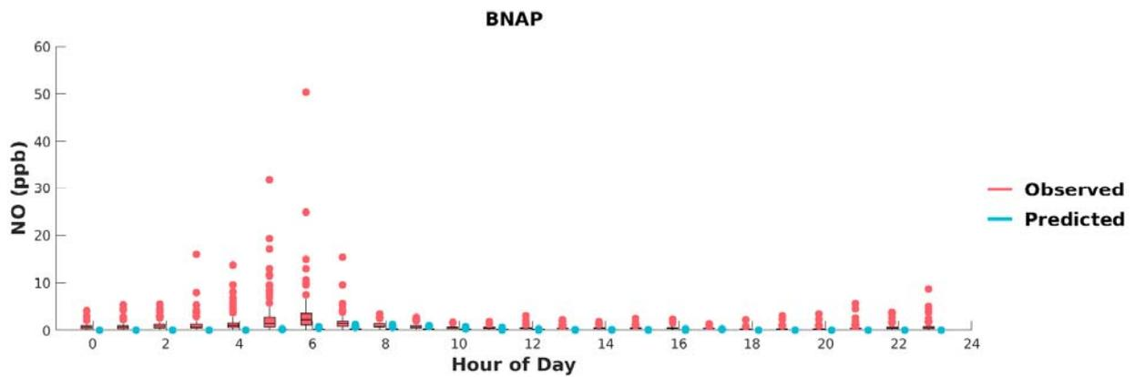
**FIGURE G-3: BOX PLOTS OF OBSERVED VS. PREDICTED HOURLY NO DURING MAY 1<sup>ST</sup> TO SEPTEMBER 30<sup>TH</sup>, 2018, AT BANNING. HORIZONTAL LINES INDICATE 25<sup>TH</sup>, 50<sup>TH</sup> (MEDIAN), AND 75<sup>TH</sup> PERCENTILES.**
