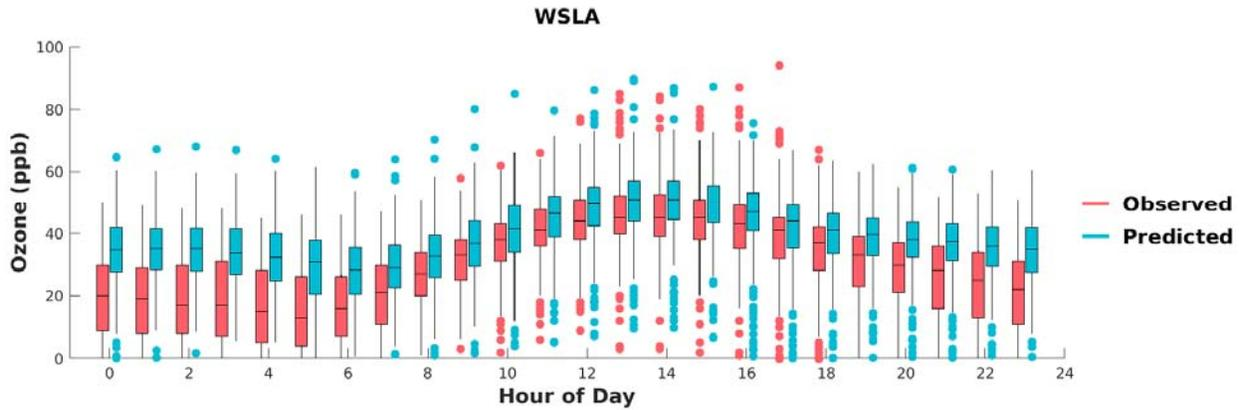
**FIGURE F-31: BOX PLOTS OF OBSERVED VS. PREDICTED HOURLY OZONE DURING MAY 1<sup>ST</sup> TO SEPTEMBER 30<sup>TH</sup>, 2018, AT WEST LOS ANGELES. HORIZONTAL LINES INDICATE 25<sup>TH</sup>, 50<sup>TH</sup> (MEDIAN), AND 75<sup>TH</sup> PERCENTILES.**
