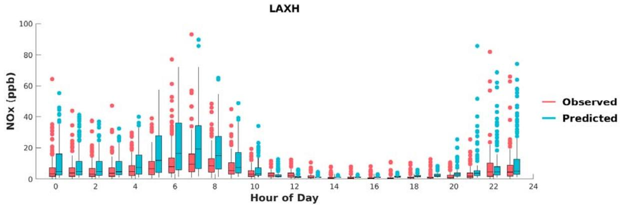
**FIGURE I-11: BOX PLOTS OF OBSERVED VS. PREDICTED HOURLY NOX DURING MAY 1<sup>ST</sup> TO SEPTEMBER 30<sup>TH</sup>, 2018, AT LAX. HORIZONTAL LINES INDICATE 25<sup>TH</sup>, 50<sup>TH</sup> (MEDIAN), AND 75<sup>TH</sup> PERCENTILES.**
