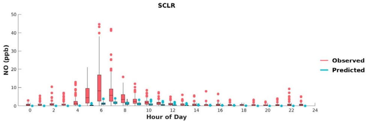
**FIGURE G-19: BOX PLOTS OF OBSERVED VS. PREDICTED HOURLY NO DURING MAY 1<sup>ST</sup> TO SEPTEMBER 30<sup>TH</sup>, 2018, AT SANTA CLARITA. HORIZONTAL LINES INDICATE 25<sup>TH</sup>, 50<sup>TH</sup> (MEDIAN), AND 75<sup>TH</sup> PERCENTILES.**
