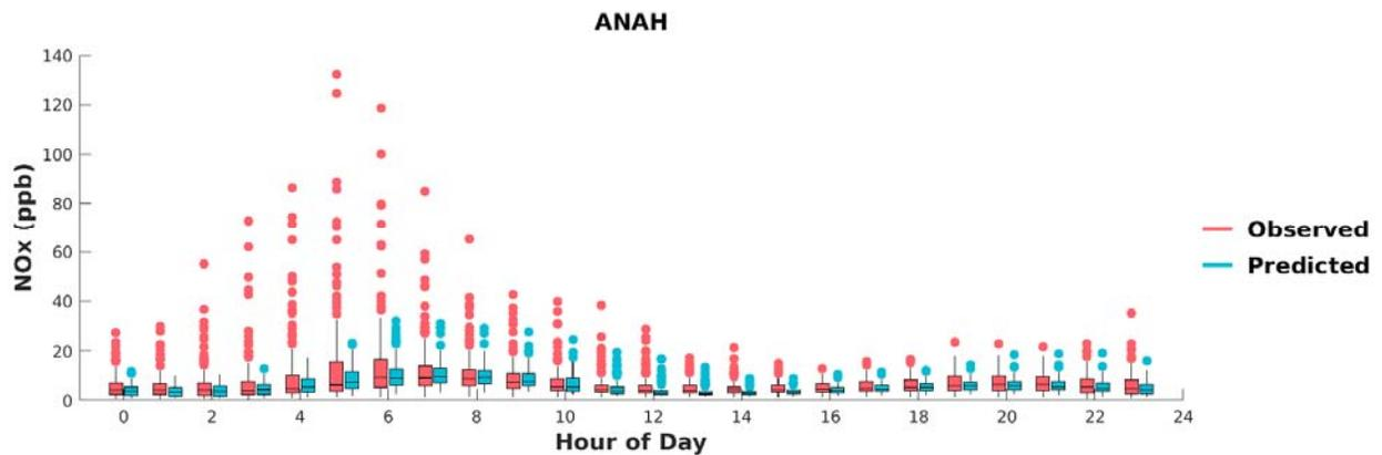
**FIGURE I-1: BOX PLOTS OF OBSERVED VS. PREDICTED HOURLY NO<sub>x</sub> DURING MAY 1<sup>ST</sup> TO SEPTEMBER 30<sup>TH</sup>, 2018, AT ANAHEIM. HORIZONTAL LINES INDICATE 25<sup>TH</sup>, 50<sup>TH</sup> (MEDIAN), AND 75<sup>TH</sup> PERCENTILES.**
