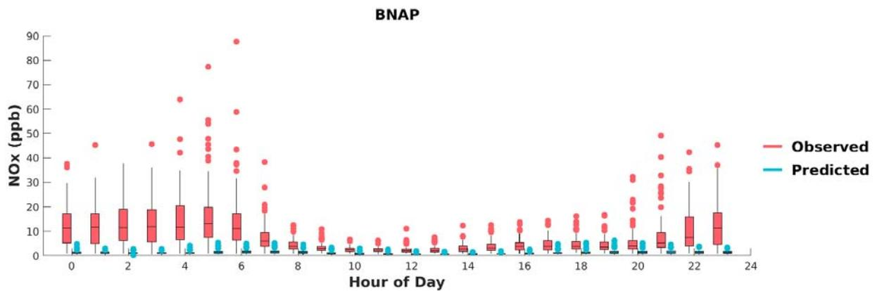
**FIGURE I-3: BOX PLOTS OF OBSERVED VS. PREDICTED HOURLY NO<sub>x</sub> DURING MAY 1<sup>ST</sup> TO SEPTEMBER 30<sup>TH</sup>, 2018, AT BANNING. HORIZONTAL LINES INDICATE 25<sup>TH</sup>, 50<sup>TH</sup> (MEDIAN), AND 75<sup>TH</sup> PERCENTILES.**
