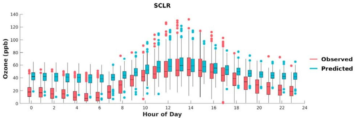
**FIGURE F-26: BOX PLOTS OF OBSERVED VS. PREDICTED HOURLY OZONE DURING MAY 1<sup>ST</sup> TO SEPTEMBER 30<sup>TH</sup>, 2018, AT SANTA CLARITA. HORIZONTAL LINES INDICATE 25<sup>TH</sup>, 50<sup>TH</sup> (MEDIAN), AND 75<sup>TH</sup> PERCENTILES.**
