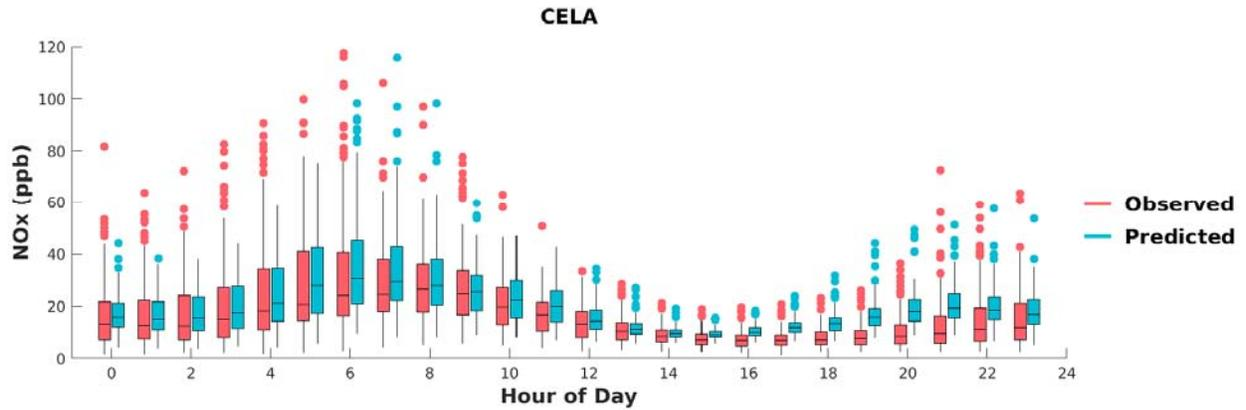
**FIGURE I-4: BOX PLOTS OF OBSERVED VS. PREDICTED HOURLY NO<sub>x</sub> DURING MAY 1<sup>ST</sup> TO SEPTEMBER 30<sup>TH</sup>, 2018, AT CENTRAL LOS ANGELES. HORIZONTAL LINES INDICATE 25<sup>TH</sup>, 50<sup>TH</sup> (MEDIAN), AND 75<sup>TH</sup> PERCENTILES.**
