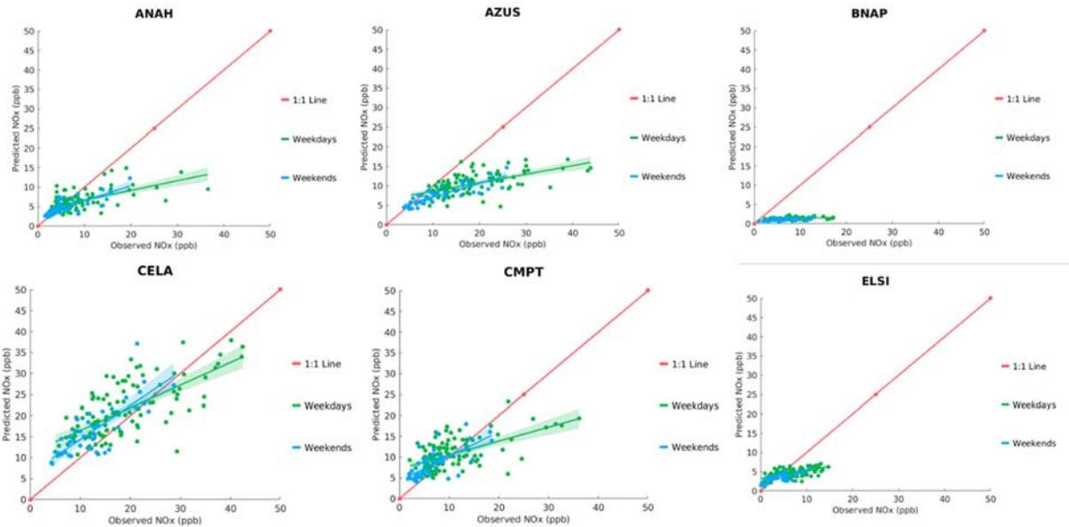
**FIGURE N-1: SCATTER PLOT OF OBSERVED VS. PREDICTED DAILY AVERAGE NO<sub>x</sub> DURING MAY 1<sup>ST</sup> TO SEPTEMBER 30<sup>TH</sup>, 2018, AT ANEHIM (ANAH), AZUSA (AZUS), BANNING (BANP), COMPTON (CMPT), CENTRAL LOS ANGELES (CELA), AND LAKE ELSINORE (ELSI). GREEN AND BLUE LINES INDICATE GENERAL LINEAR MODEL FIT WITH 95% CONFIDENCE INTERVAL (SHADED AREA). THE RED LINE INDICATES 1:1 LINE.**
