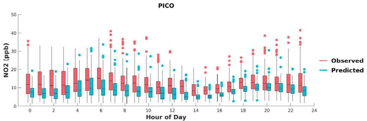
**FIGURE H-14: BOX PLOTS OF OBSERVED VS. PREDICTED HOURLY NO<sub>2</sub> DURING MAY 1<sup>ST</sup> TO SEPTEMBER 30<sup>TH</sup>, 2018, AT PICO RIVERO. HORIZONTAL LINES INDICATE 25<sup>TH</sup>, 50<sup>TH</sup> (MEDIAN), AND 75<sup>TH</sup> PERCENTILES.**
