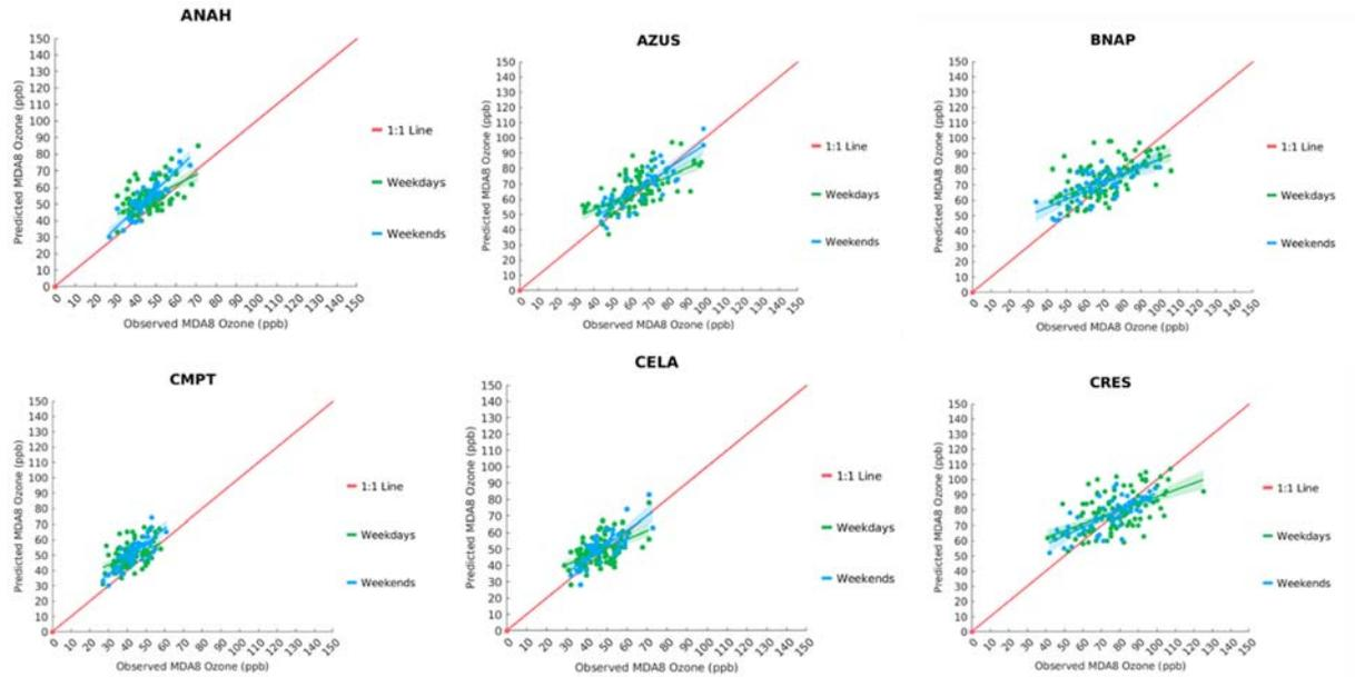
**FIGURE K-1: SCATTER PLOT OF OBSERVED VS. PREDICTED MDA8 OZONE DURING MAY 1<sup>ST</sup> TO SEPTEMBER 30<sup>TH</sup>, 2018, AT ANEHIM (ANAH), AZUSA (AZUS), BANNING (BANP), COMPTON (CMPT), CENTRAL LOS ANGELES (CELA), AND CRESTLINE (CRES). GREEN AND BLUE LINES INDICATE GENERAL LINEAR MODEL FIT WITH 95% CONFIDENCE INTERVAL (SHADED AREA). THE RED LINE INDICATES 1:1 LINE.**
