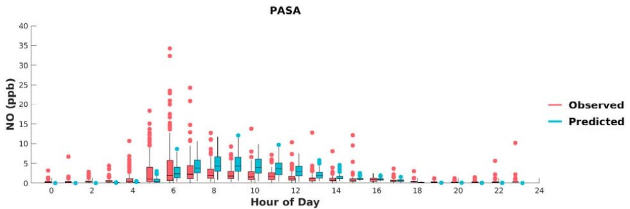
**FIGURE G-13: BOX PLOTS OF OBSERVED VS. PREDICTED HOURLY NO DURING MAY 1<sup>ST</sup> TO SEPTEMBER 30<sup>TH</sup>, 2018, AT PASADENA. HORIZONTAL LINES INDICATE 25<sup>TH</sup>, 50<sup>TH</sup> (MEDIAN), AND 75<sup>TH</sup> PERCENTILES.**
