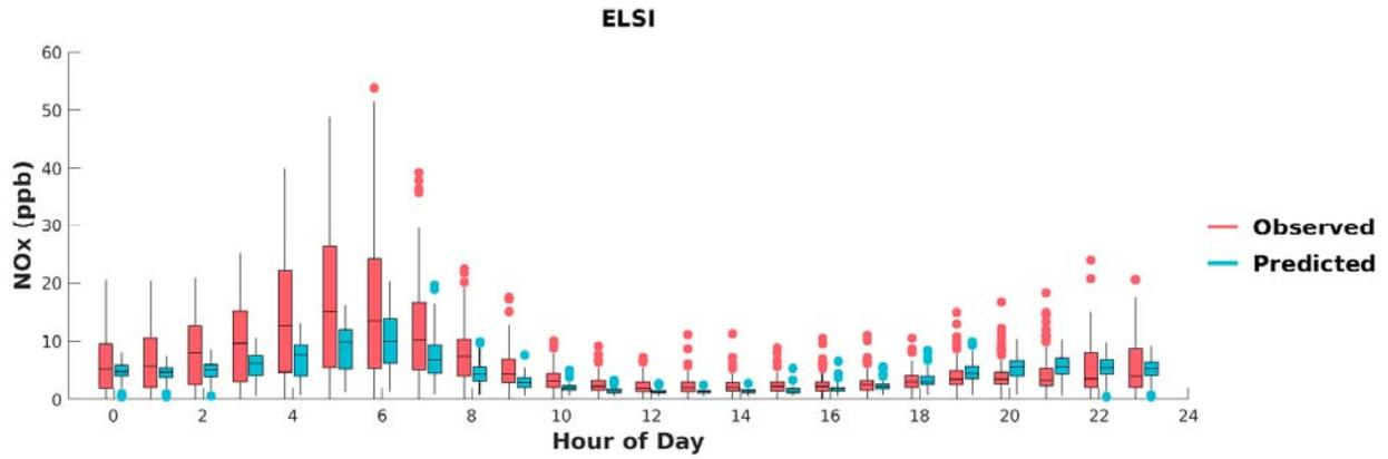
**FIGURE I-6: BOX PLOTS OF OBSERVED VS. PREDICTED HOURLY NOX DURING MAY 1<sup>ST</sup> TO SEPTEMBER 30<sup>TH</sup>, 2018, AT LAKE ELSINORE. HORIZONTAL LINES INDICATE 25<sup>TH</sup>, 50<sup>TH</sup> (MEDIAN), AND 75<sup>TH</sup> PERCENTILES.**
