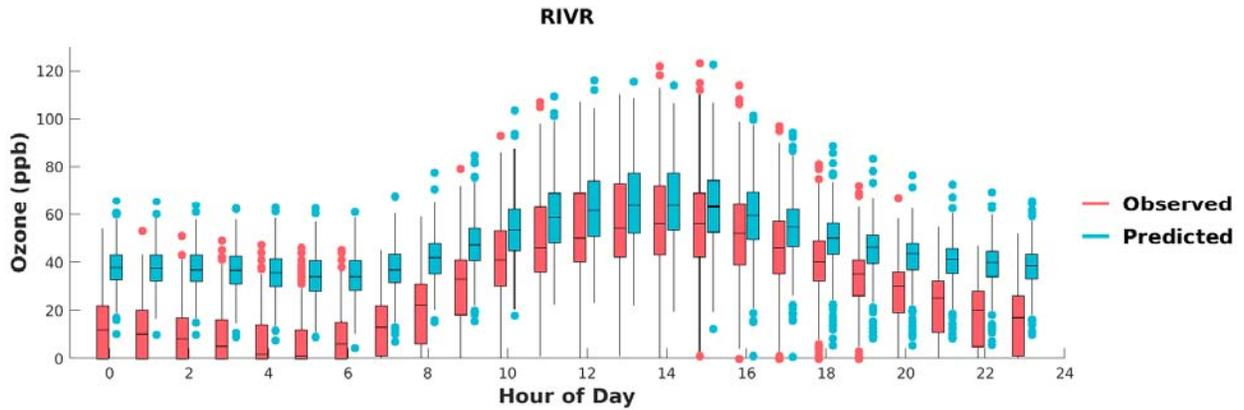
**FIGURE F-25: BOX PLOTS OF OBSERVED VS. PREDICTED HOURLY OZONE DURING MAY 1<sup>ST</sup> TO SEPTEMBER 30<sup>TH</sup>, 2018, AT RIVERSIDE. HORIZONTAL LINES INDICATE 25<sup>TH</sup>, 50<sup>TH</sup> (MEDIAN), AND 75<sup>TH</sup> PERCENTILES.**
