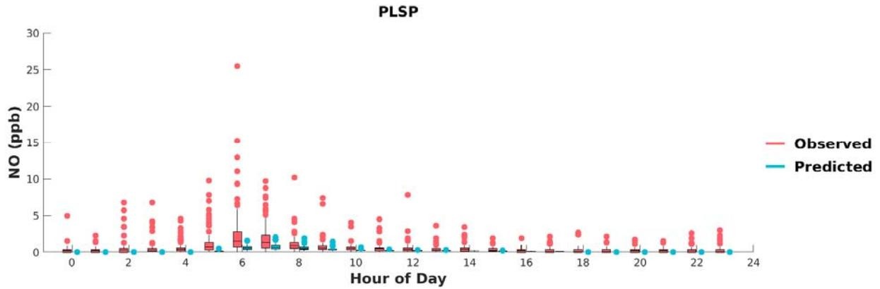
**FIGURE G-16: BOX PLOTS OF OBSERVED VS. PREDICTED HOURLY NO DURING MAY 1<sup>ST</sup> TO SEPTEMBER 30<sup>TH</sup>, 2018, AT PALM SPRINGS. HORIZONTAL LINES INDICATE 25<sup>TH</sup>, 50<sup>TH</sup> (MEDIAN), AND 75<sup>TH</sup> PERCENTILES.**
