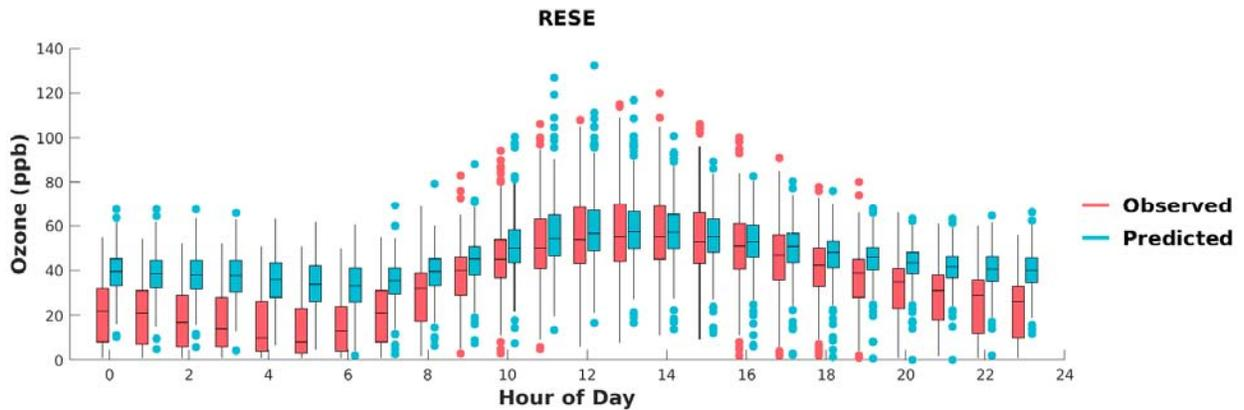
**FIGURE F-24: BOX PLOTS OF OBSERVED VS. PREDICTED HOURLY OZONE DURING MAY 1<sup>ST</sup> TO SEPTEMBER 30<sup>TH</sup>, 2018, AT RESEDA. HORIZONTAL LINES INDICATE 25<sup>TH</sup>, 50<sup>TH</sup> (MEDIAN), AND 75<sup>TH</sup> PERCENTILES.**
