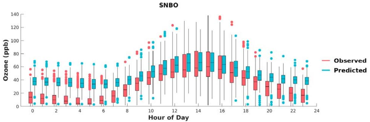
**FIGURE F-28: BOX PLOTS OF OBSERVED VS. PREDICTED HOURLY OZONE DURING MAY 1<sup>ST</sup> TO SEPTEMBER 30<sup>TH</sup>, 2018, AT SAN BERNARDINO. HORIZONTAL LINES INDICATE 25<sup>TH</sup>, 50<sup>TH</sup> (MEDIAN), AND 75<sup>TH</sup> PERCENTILES.**
