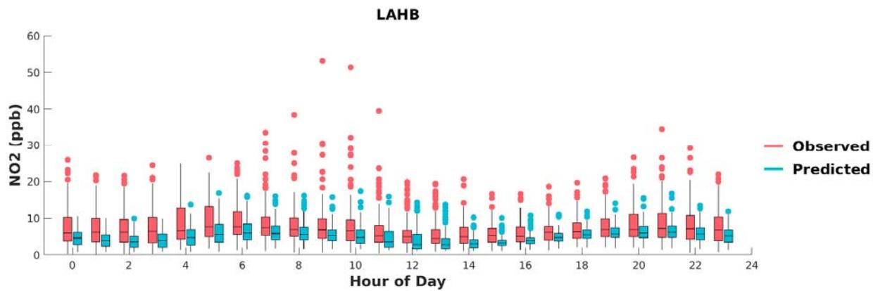
**FIGURE H-10: BOX PLOTS OF OBSERVED VS. PREDICTED HOURLY NO<sub>2</sub> DURING MAY 1<sup>ST</sup> TO SEPTEMBER 30<sup>TH</sup>, 2018, AT LA HABRA. HORIZONTAL LINES INDICATE 25<sup>TH</sup>, 50<sup>TH</sup> (MEDIAN), AND 75<sup>TH</sup> PERCENTILES.**
