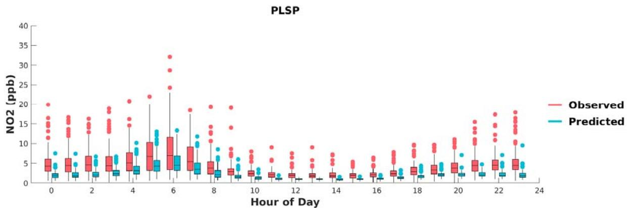
FIGURE H-16: BOX PLOTS OF OBSERVED VS. PREDICTED HOURLY NO<sub>2</sub> DURING MAY 1<sup>ST</sup> TO SEPTEMBER 30<sup>TH</sup>, 2018, AT PALM SPRINGS. HORIZONTAL LINES INDICATE 25<sup>TH</sup>, 50<sup>TH</sup> (MEDIAN), AND 75<sup>TH</sup> PERCENTILES.
