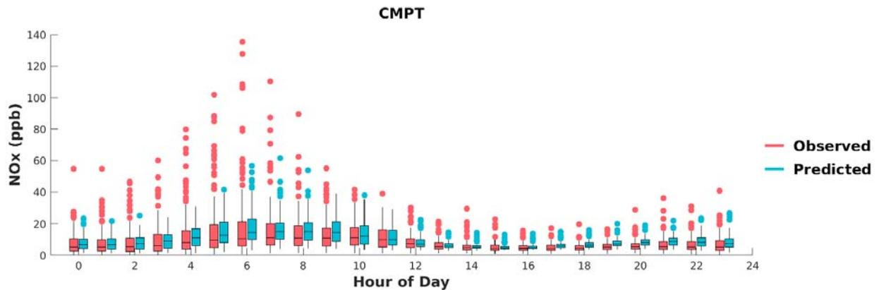
**FIGURE I-5: BOX PLOTS OF OBSERVED VS. PREDICTED HOURLY NO<sub>x</sub> DURING MAY 1<sup>ST</sup> TO SEPTEMBER 30<sup>TH</sup>, 2018, AT COMPTON. HORIZONTAL LINES INDICATE 25<sup>TH</sup>, 50<sup>TH</sup> (MEDIAN), AND 75<sup>TH</sup> PERCENTILES.**
