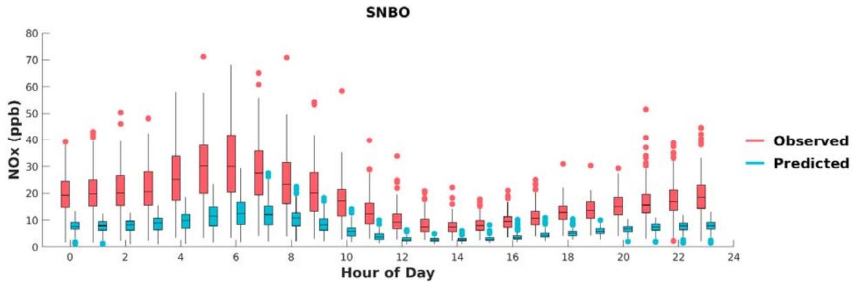
**FIGURE I-21: BOX PLOTS OF OBSERVED VS. PREDICTED HOURLY NOx DURING MAY 1<sup>ST</sup> TO SEPTEMBER 30<sup>TH</sup>, 2018, AT SAN BERNARDINO. HORIZONTAL LINES INDICATE 25<sup>TH</sup>, 50<sup>TH</sup> (MEDIAN), AND 75<sup>TH</sup> PERCENTILES.**
