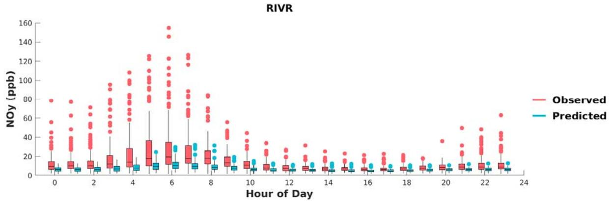
**FIGURE J-1: BOX PLOTS OF OBSERVED VS. PREDICTED HOURLY NO<sub>y</sub> DURING MAY 1<sup>ST</sup> TO SEPTEMBER 30<sup>TH</sup>, 2018, AT RIVERSIDE. HORIZONTAL LINES INDICATE 25<sup>TH</sup>, 50<sup>TH</sup> (MEDIAN), AND 75<sup>TH</sup> PERCENTILES.**
