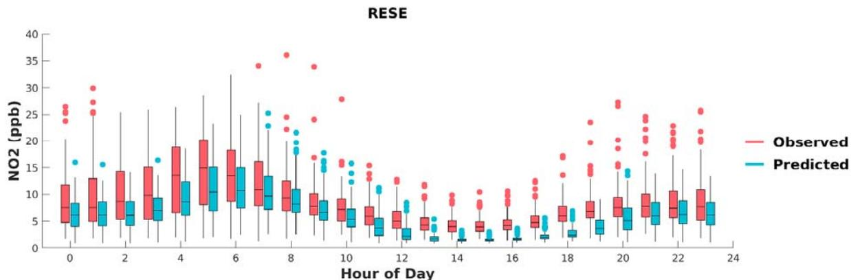
**FIGURE H-17: BOX PLOTS OF OBSERVED VS. PREDICTED HOURLY NO<sub>2</sub> DURING MAY 1<sup>ST</sup> TO SEPTEMBER 30<sup>TH</sup>, 2018, AT RESEDA. HORIZONTAL LINES INDICATE 25<sup>TH</sup>, 50<sup>TH</sup> (MEDIAN), AND 75<sup>TH</sup> PERCENTILES.**
