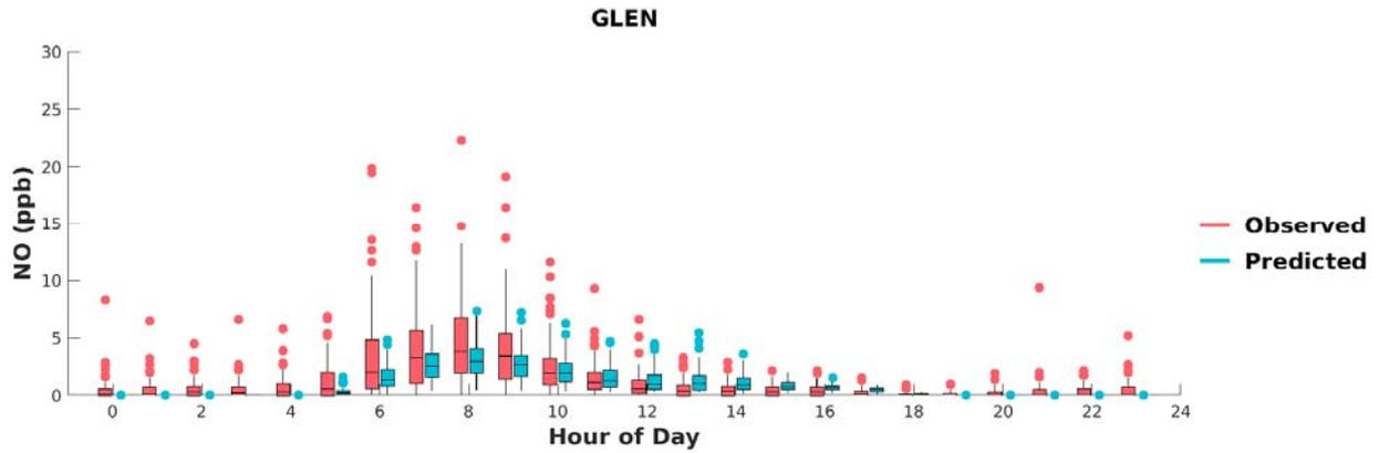
**FIGURE G-8: BOX PLOTS OF OBSERVED VS. PREDICTED HOURLY NO DURING MAY 1<sup>ST</sup> TO SEPTEMBER 30<sup>TH</sup>, 2018, AT GLENDORA. HORIZONTAL LINES INDICATE 25<sup>TH</sup>, 50<sup>TH</sup> (MEDIAN), AND 75<sup>TH</sup> PERCENTILES.**
