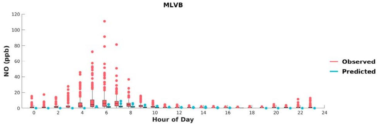
**FIGURE G-12: BOX PLOTS OF OBSERVED VS. PREDICTED HOURLY NO DURING MAY 1<sup>ST</sup> TO SEPTEMBER 30<sup>TH</sup>, 2018, AT MIRA LOMA VAN BUREN. HORIZONTAL LINES INDICATE 25<sup>TH</sup>, 50<sup>TH</sup> (MEDIAN), AND 75<sup>TH</sup> PERCENTILES.**
