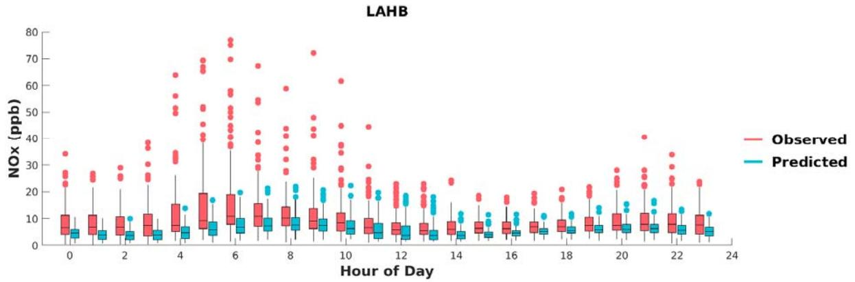
**FIGURE I-10: BOX PLOTS OF OBSERVED VS. PREDICTED HOURLY NOX DURING MAY 1<sup>ST</sup> TO SEPTEMBER 30<sup>TH</sup>, 2018, AT LA HABRA. HORIZONTAL LINES INDICATE 25<sup>TH</sup>, 50<sup>TH</sup> (MEDIAN), AND 75<sup>TH</sup> PERCENTILES.**
