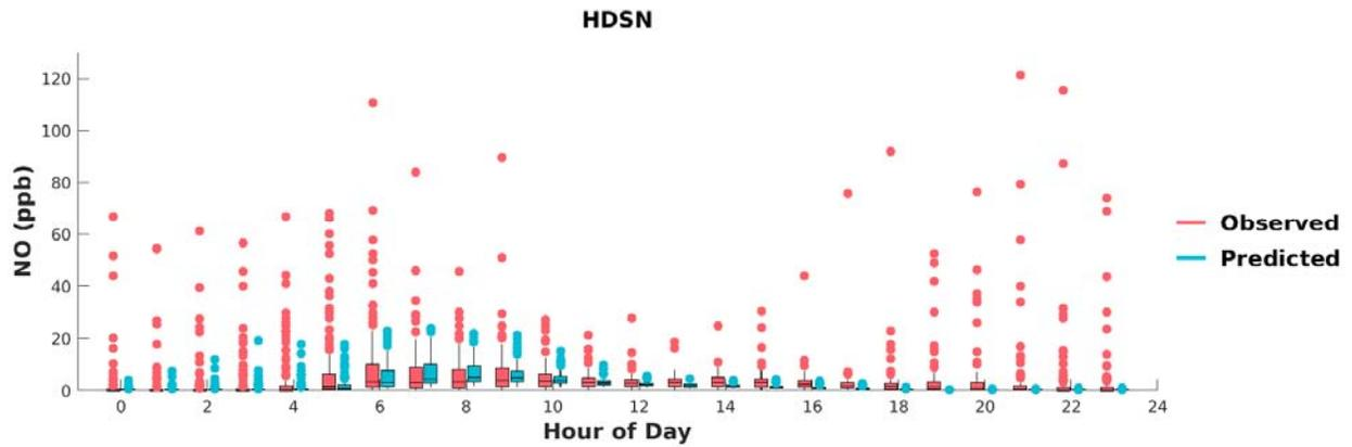
**FIGURE G-9: BOX PLOTS OF OBSERVED VS. PREDICTED HOURLY NO DURING MAY 1<sup>ST</sup> TO SEPTEMBER 30<sup>TH</sup>, 2018, AT HUDSON. HORIZONTAL LINES INDICATE 25<sup>TH</sup>, 50<sup>TH</sup> (MEDIAN), AND 75<sup>TH</sup> PERCENTILES.**
