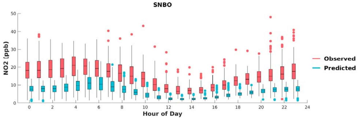
**FIGURE H-21: BOX PLOTS OF OBSERVED VS. PREDICTED HOURLY NO<sub>2</sub> DURING MAY 1<sup>ST</sup> TO SEPTEMBER 30<sup>TH</sup>, 2018, AT SAN BERNARDINO. HORIZONTAL LINES INDICATE 25<sup>TH</sup>, 50<sup>TH</sup> (MEDIAN), AND 75<sup>TH</sup> PERCENTILES.**
