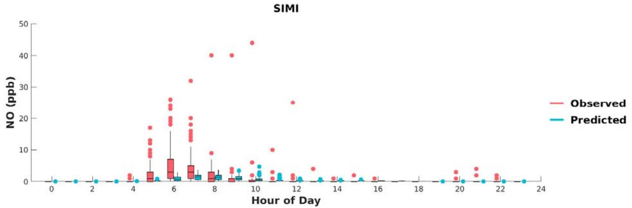
**FIGURE G-20: BOX PLOTS OF OBSERVED VS. PREDICTED HOURLY NO DURING MAY 1<sup>ST</sup> TO SEPTEMBER 30<sup>TH</sup>, 2018, AT SIMI VALLEY. HORIZONTAL LINES INDICATE 25<sup>TH</sup>, 50<sup>TH</sup> (MEDIAN), AND 75<sup>TH</sup> PERCENTILES.**
