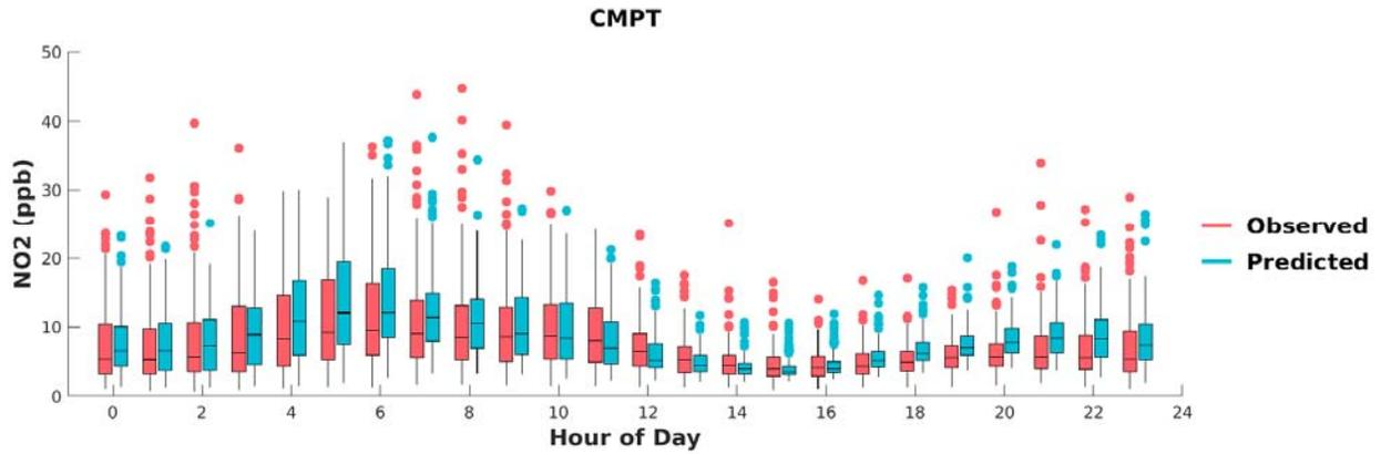
**FIGURE H-5: BOX PLOTS OF OBSERVED VS. PREDICTED HOURLY NO<sub>2</sub> DURING MAY 1<sup>ST</sup> TO SEPTEMBER 30<sup>TH</sup>, 2018, AT COMPTON. HORIZONTAL LINES INDICATE 25<sup>TH</sup>, 50<sup>TH</sup> (MEDIAN), AND 75<sup>TH</sup> PERCENTILES.**
