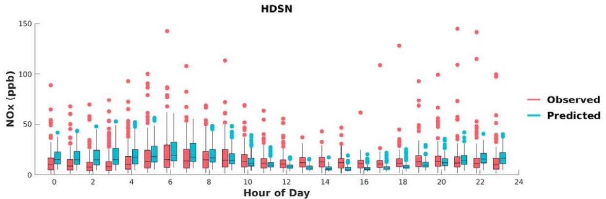
**FIGURE I-9: BOX PLOTS OF OBSERVED VS. PREDICTED HOURLY NOX DURING MAY 1<sup>ST</sup> TO SEPTEMBER 30<sup>TH</sup>, 2018, AT HUDSON. HORIZONTAL LINES INDICATE 25<sup>TH</sup>, 50<sup>TH</sup> (MEDIAN), AND 75<sup>TH</sup> PERCENTILES.**
