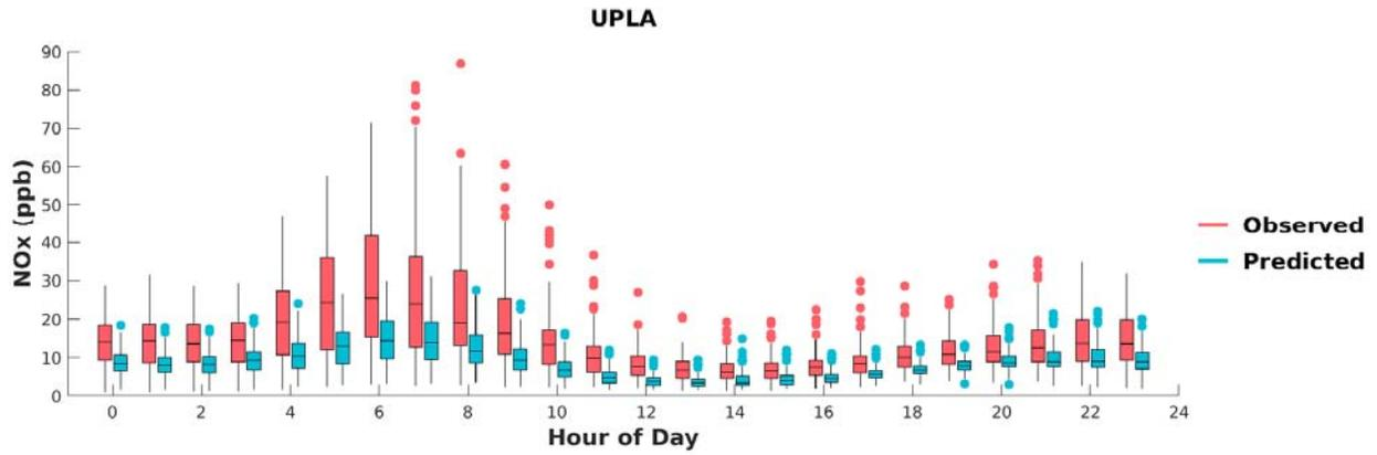
**FIGURE I-22: BOX PLOTS OF OBSERVED VS. PREDICTED HOURLY NOx DURING MAY 1<sup>ST</sup> TO SEPTEMBER 30<sup>TH</sup>, 2018, AT UPLAND. HORIZONTAL LINES INDICATE 25<sup>TH</sup>, 50<sup>TH</sup> (MEDIAN), AND 75<sup>TH</sup> PERCENTILES.**
