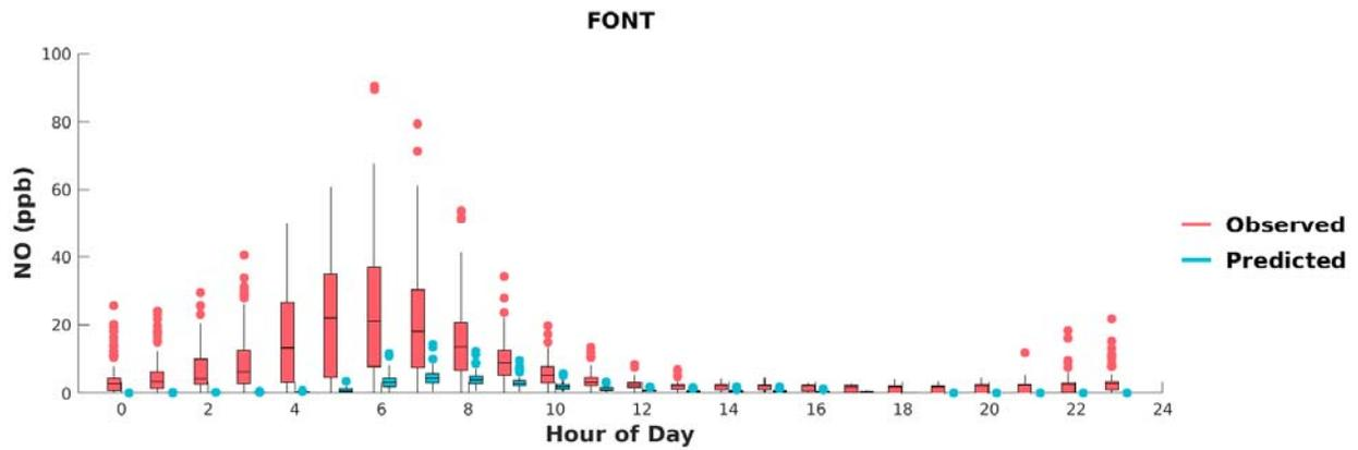
**FIGURE G-7: BOX PLOTS OF OBSERVED VS. PREDICTED HOURLY NO DURING MAY 1<sup>ST</sup> TO SEPTEMBER 30<sup>TH</sup>, 2018, AT FONTANA. HORIZONTAL LINES INDICATE 25<sup>TH</sup>, 50<sup>TH</sup> (MEDIAN), AND 75<sup>TH</sup> PERCENTILES.**
