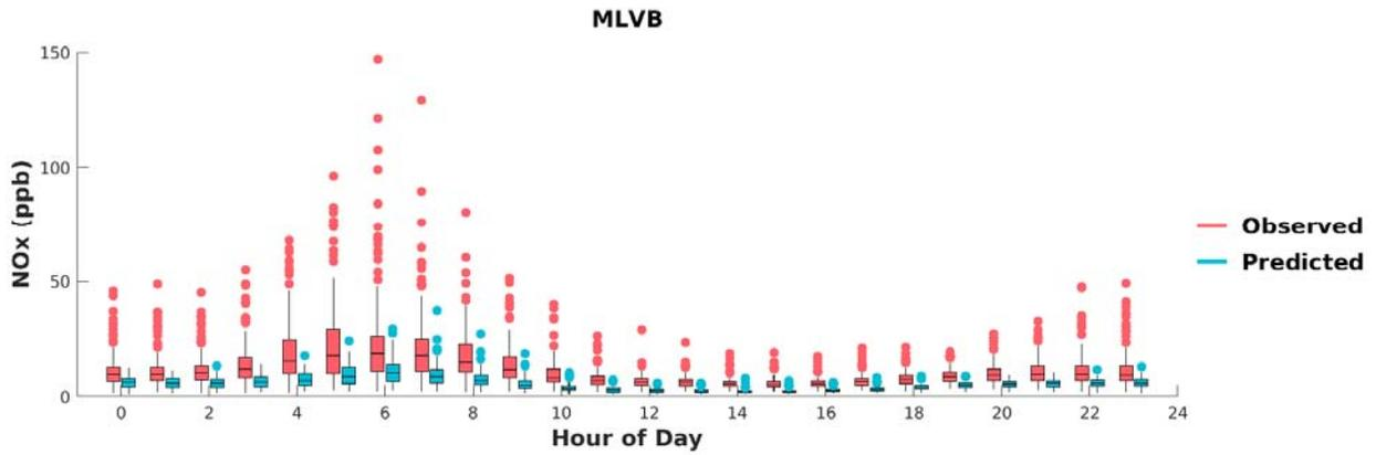
**FIGURE I-12: BOX PLOTS OF OBSERVED VS. PREDICTED HOURLY NOX DURING MAY 1<sup>ST</sup> TO SEPTEMBER 30<sup>TH</sup>, 2018, AT MIRA LOMA VAN BUREN. HORIZONTAL LINES INDICATE 25<sup>TH</sup>, 50<sup>TH</sup> (MEDIAN), AND 75<sup>TH</sup> PERCENTILES.**
