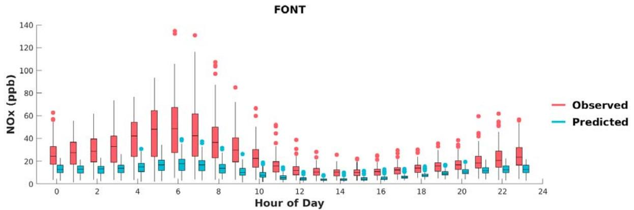
**FIGURE I-7: BOX PLOTS OF OBSERVED VS. PREDICTED HOURLY NOX DURING MAY 1<sup>ST</sup> TO SEPTEMBER 30<sup>TH</sup>, 2018, AT FONTANA. HORIZONTAL LINES INDICATE 25<sup>TH</sup>, 50<sup>TH</sup> (MEDIAN), AND 75<sup>TH</sup> PERCENTILES.**
