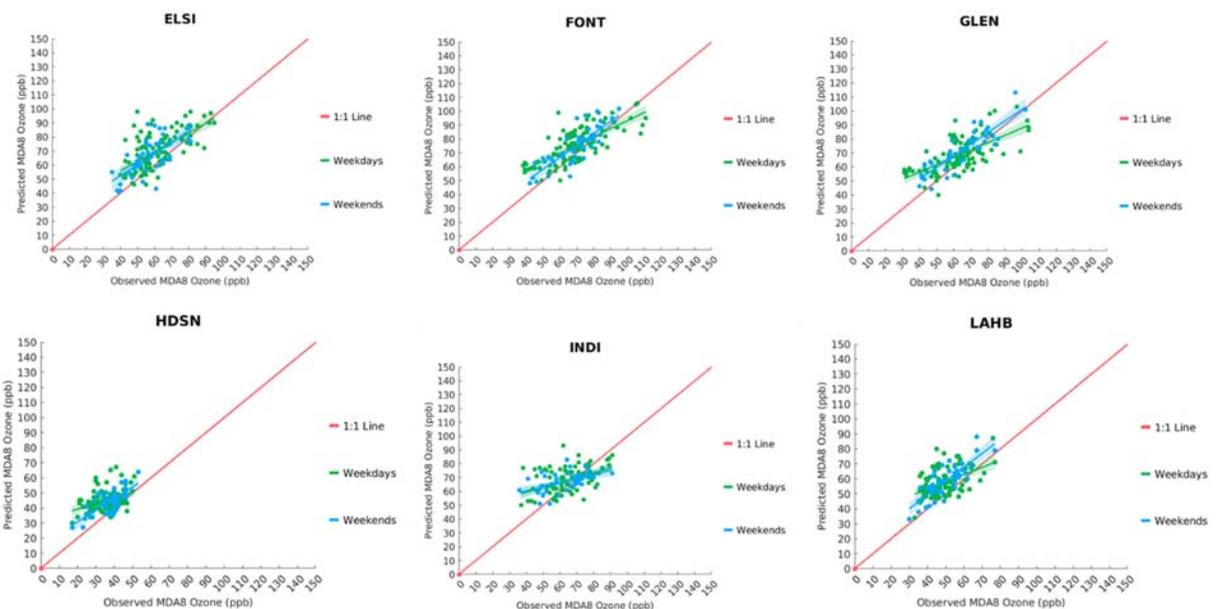
**FIGURE K-2: SCATTER PLOT OF OBSERVED VS. PREDICTED MDA8 OZONE DURING MAY 1<sup>ST</sup> TO SEPTEMBER 30<sup>TH</sup>, 2018, AT LAKE ELSINORE (ELSI), FONTANA (FONT), GLENDORA (GLEN), HUDSON (HDSN), INDIO (INDI), AND LA HABRA (LAHB). GREEN AND BLUE LINES INDICATE GENERAL LINEAR MODEL FIT WITH 95% CONFIDENCE INTERVAL (SHADED AREA). THE RED LINE INDICATES 1:1 LINE.**
