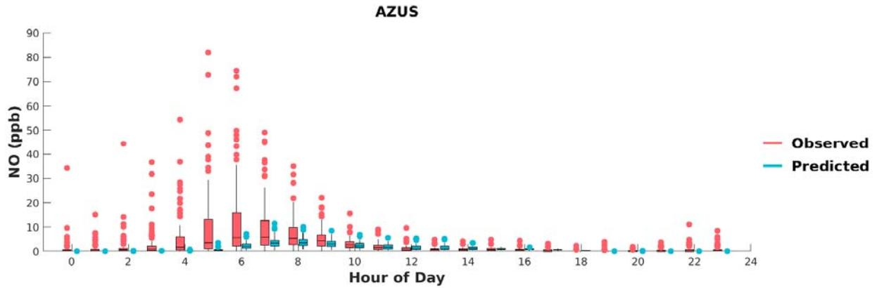
**FIGURE G-2: BOX PLOTS OF OBSERVED VS. PREDICTED HOURLY NO DURING MAY 1<sup>ST</sup> TO SEPTEMBER 30<sup>TH</sup>, 2018, AT AZUSA. HORIZONTAL LINES INDICATE 25<sup>TH</sup>, 50<sup>TH</sup> (MEDIAN), AND 75<sup>TH</sup> PERCENTILES.**
