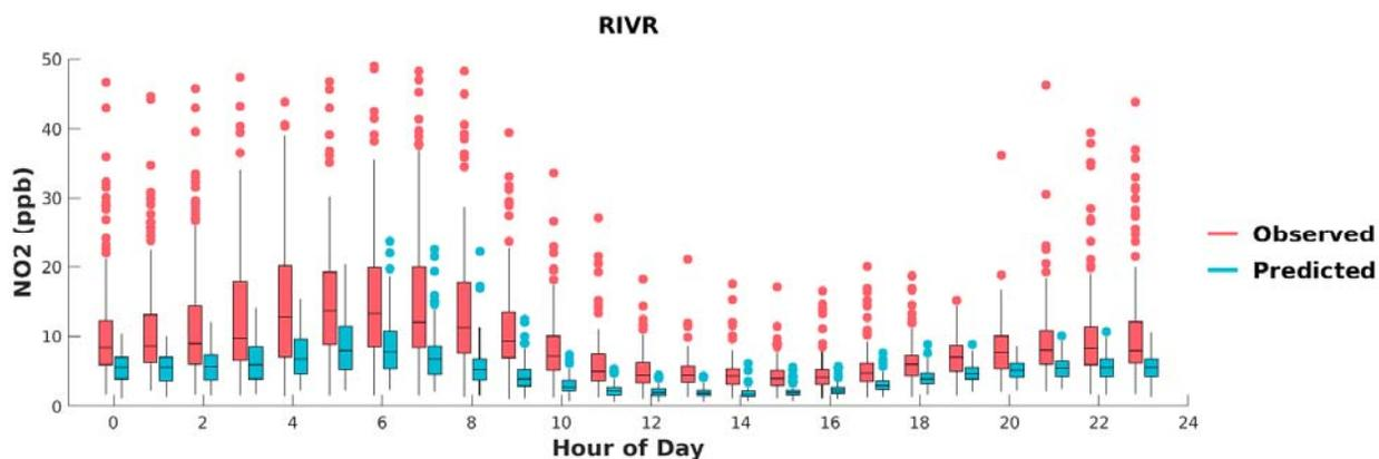
**FIGURE H-18: BOX PLOTS OF OBSERVED VS. PREDICTED HOURLY NO<sub>2</sub> DURING MAY 1<sup>ST</sup> TO SEPTEMBER 30<sup>TH</sup>, 2018, AT RIVERSIDE. HORIZONTAL LINES INDICATE 25<sup>TH</sup>, 50<sup>TH</sup> (MEDIAN), AND 75<sup>TH</sup> PERCENTILES.**
