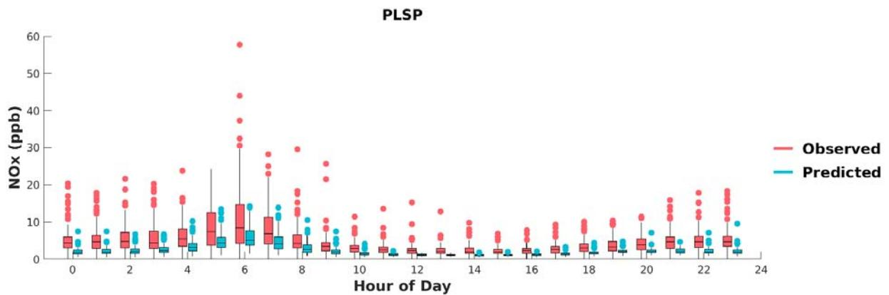
**FIGURE I-15: BOX PLOTS OF OBSERVED VS. PREDICTED HOURLY NOx DURING MAY 1<sup>ST</sup> TO SEPTEMBER 30<sup>TH</sup>, 2018, AT PALM SPRINGS. HORIZONTAL LINES INDICATE 25<sup>TH</sup>, 50<sup>TH</sup> (MEDIAN), AND 75<sup>TH</sup> PERCENTILES.**
