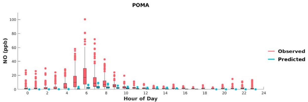
**FIGURE G-15: BOX PLOTS OF OBSERVED VS. PREDICTED HOURLY NO DURING MAY 1<sup>ST</sup> TO SEPTEMBER 30<sup>TH</sup>, 2018, AT POMONA. HORIZONTAL LINES INDICATE 25<sup>TH</sup>, 50<sup>TH</sup> (MEDIAN), AND 75<sup>TH</sup> PERCENTILES.**
