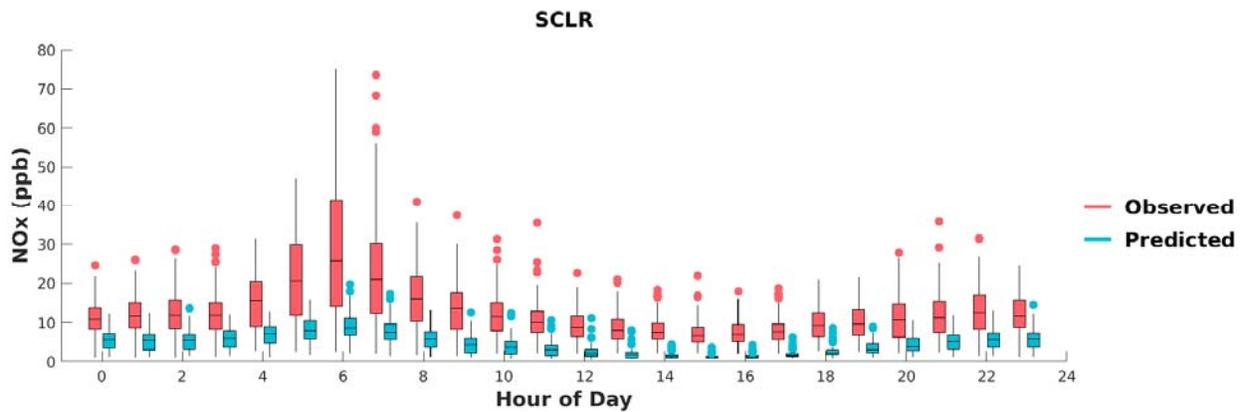
**FIGURE I-19: BOX PLOTS OF OBSERVED VS. PREDICTED HOURLY NOX DURING MAY 1<sup>ST</sup> TO SEPTEMBER 30<sup>TH</sup>, 2018, AT SANTA CLARITA. HORIZONTAL LINES INDICATE 25<sup>TH</sup>, 50<sup>TH</sup> (MEDIAN), AND 75<sup>TH</sup> PERCENTILES.**
