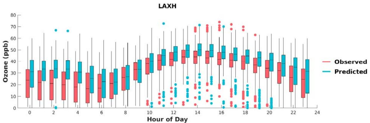
**FIGURE F-14: BOX PLOTS OF OBSERVED VS. PREDICTED HOURLY OZONE DURING MAY 1<sup>ST</sup> TO SEPTEMBER 30<sup>TH</sup>, 2018, AT LAX. HORIZONTAL LINES INDICATE 25<sup>TH</sup>, 50<sup>TH</sup> (MEDIAN), AND 75<sup>TH</sup> PERCENTILES.**
