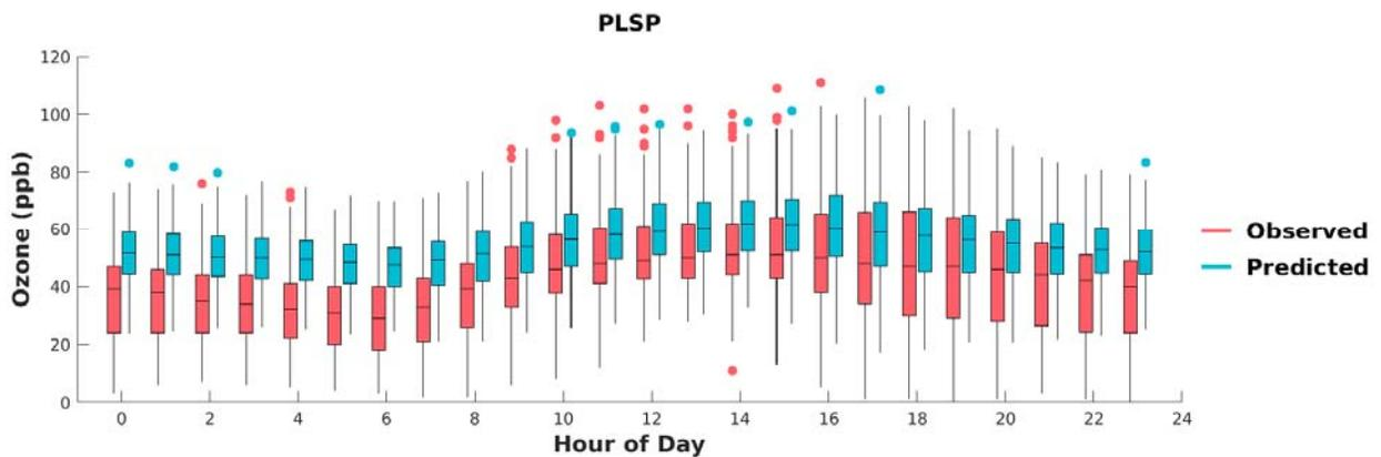
**FIGURE F-22: BOX PLOTS OF OBSERVED VS. PREDICTED HOURLY OZONE DURING MAY 1<sup>ST</sup> TO SEPTEMBER 30<sup>TH</sup>, 2018, AT PALM SPRINGS. HORIZONTAL LINES INDICATE 25<sup>TH</sup>, 50<sup>TH</sup> (MEDIAN), AND 75<sup>TH</sup> PERCENTILES.**
