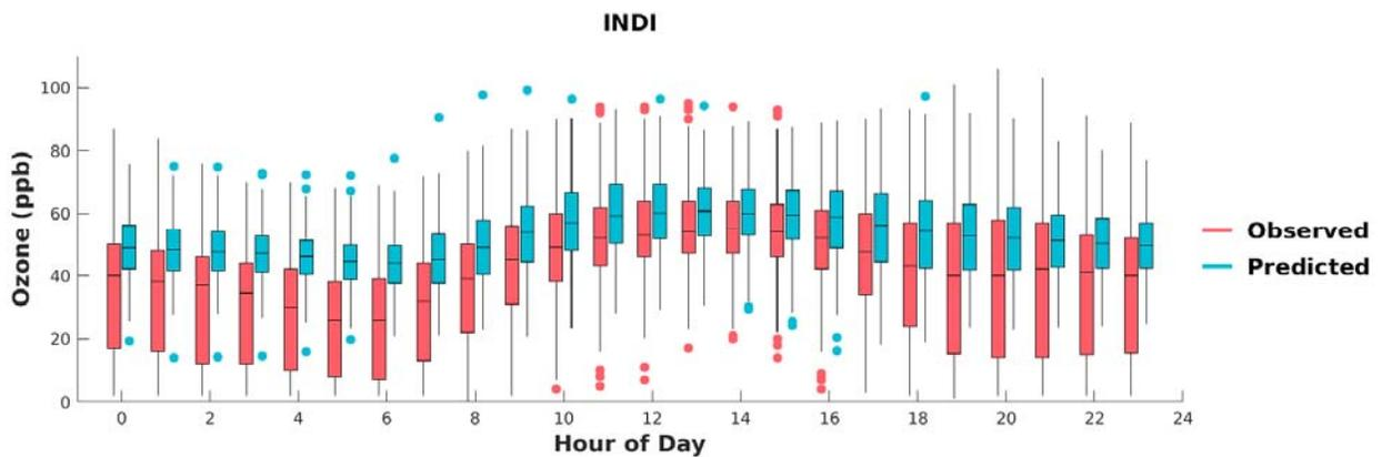
**FIGURE F-12: BOX PLOTS OF OBSERVED VS. PREDICTED HOURLY OZONE DURING MAY 1<sup>ST</sup> TO SEPTEMBER 30<sup>TH</sup>, 2018, AT INDIIO. HORIZONTAL LINES INDICATE 25<sup>TH</sup>, 50<sup>TH</sup> (MEDIAN), AND 75<sup>TH</sup> PERCENTILES.**
