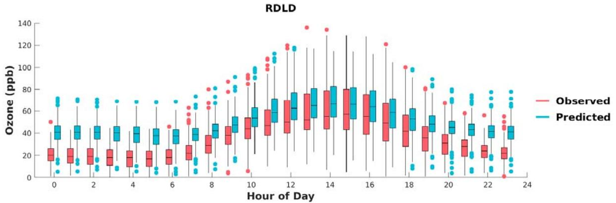
**FIGURE F-23: BOX PLOTS OF OBSERVED VS. PREDICTED HOURLY OZONE DURING MAY 1<sup>ST</sup> TO SEPTEMBER 30<sup>TH</sup>, 2018, AT REDLANDS. HORIZONTAL LINES INDICATE 25<sup>TH</sup>, 50<sup>TH</sup> (MEDIAN), AND 75<sup>TH</sup> PERCENTILES.**
