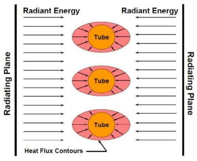
Figure 1-12 Heat transfer for a double fired process heater.
