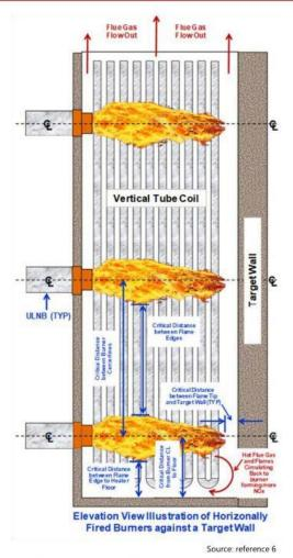
Figure 1-9 Burner firing towards a target wall.
