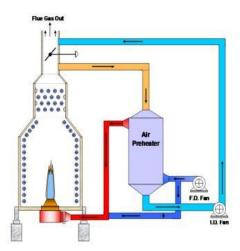
Figure 1-16 Balanced draft cabin heater.
