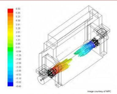
Figure 1-8 CFD model of horizontal fired cabin heater.
