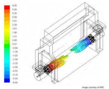
Figure 2-4 CFD model of horizontal fired cabin heater.
