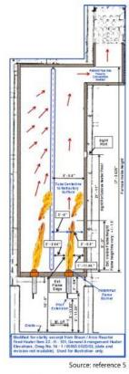
Figure 2-2 Illustration of flame impingement on process heater tubes.
