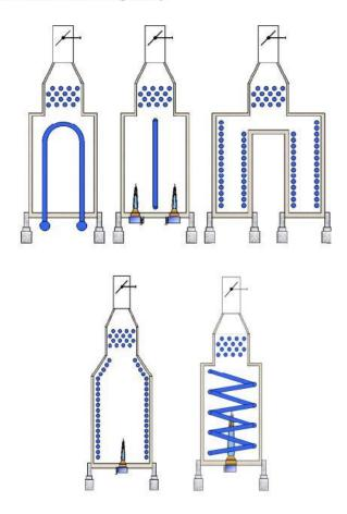
Figure 1-10 Process coil and burner orientations.
