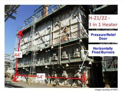
Figure 1-7 Horizontal fired "3-in-1" box heater.
