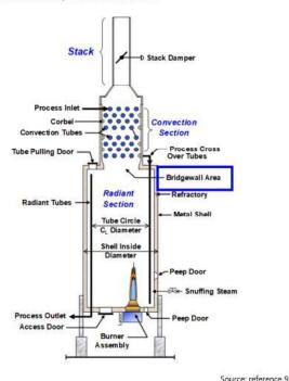
Figure 1-2 Areas and components of a refinery process heater.
