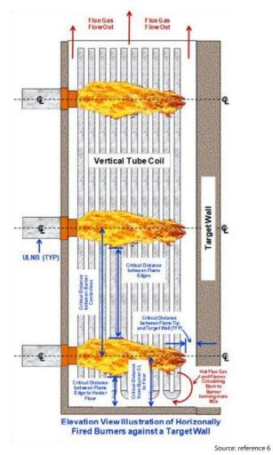
Figure 2-3 Burner firing towards a target wall.
