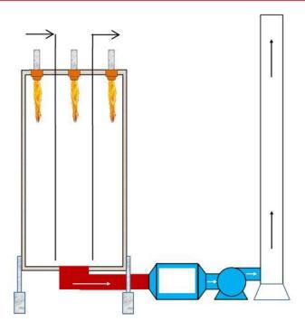
Figure 1-6 Downward fired cabin heater illustration
