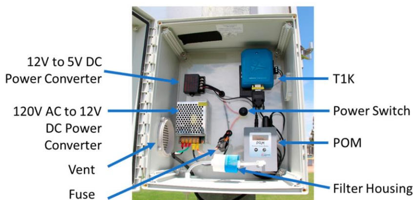
Figure 1. Ozone sensor node with labeled components.
