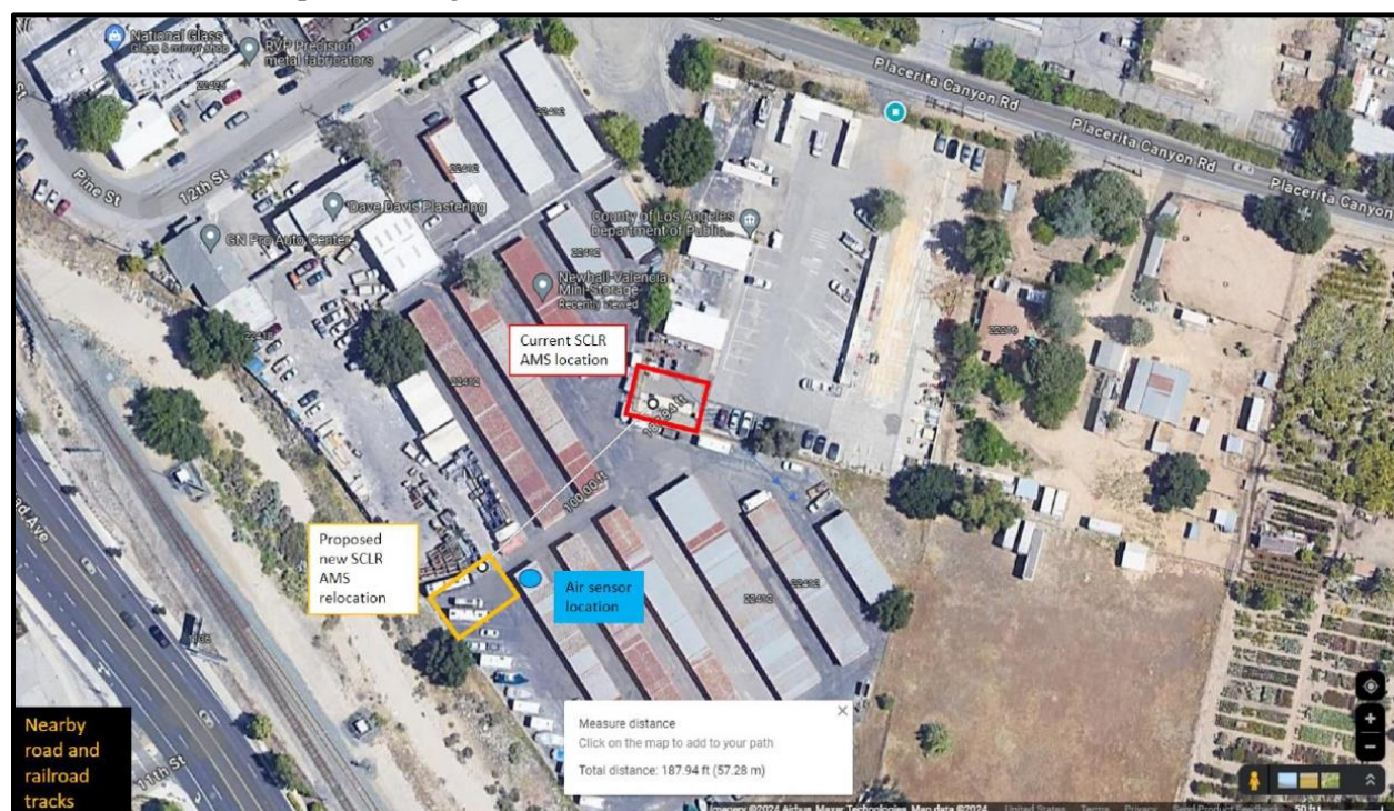
Figure 1: Map view of existing site area and major cross streets. Existing AMS is outlined in red and proposed new site is outlined in yellow. The blue dot represents the proposed air sensor deployment location, with the two sites being 190 feet apart.
