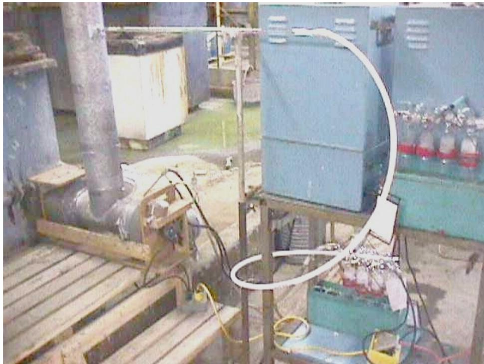
Figure 4 – Photograph of Chromium Sampling System.
