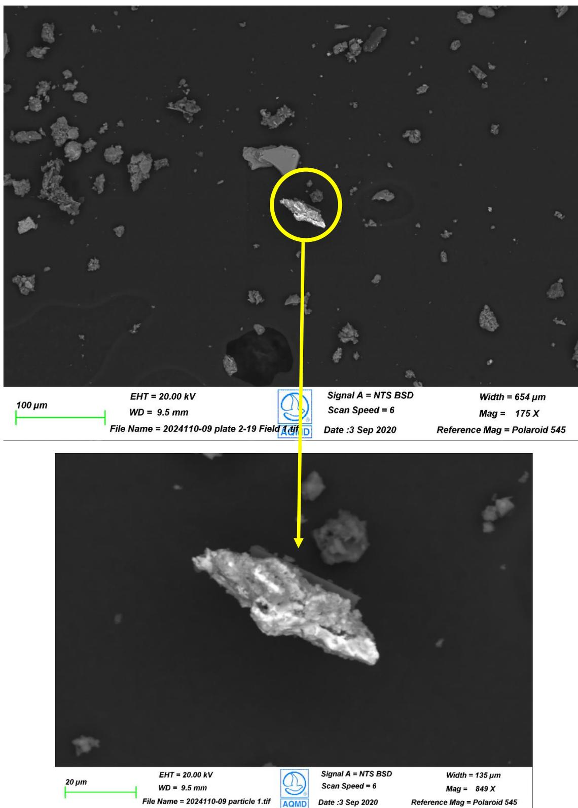
**Figure 4.** Westside #2: Amorphous Pb containing particle.
