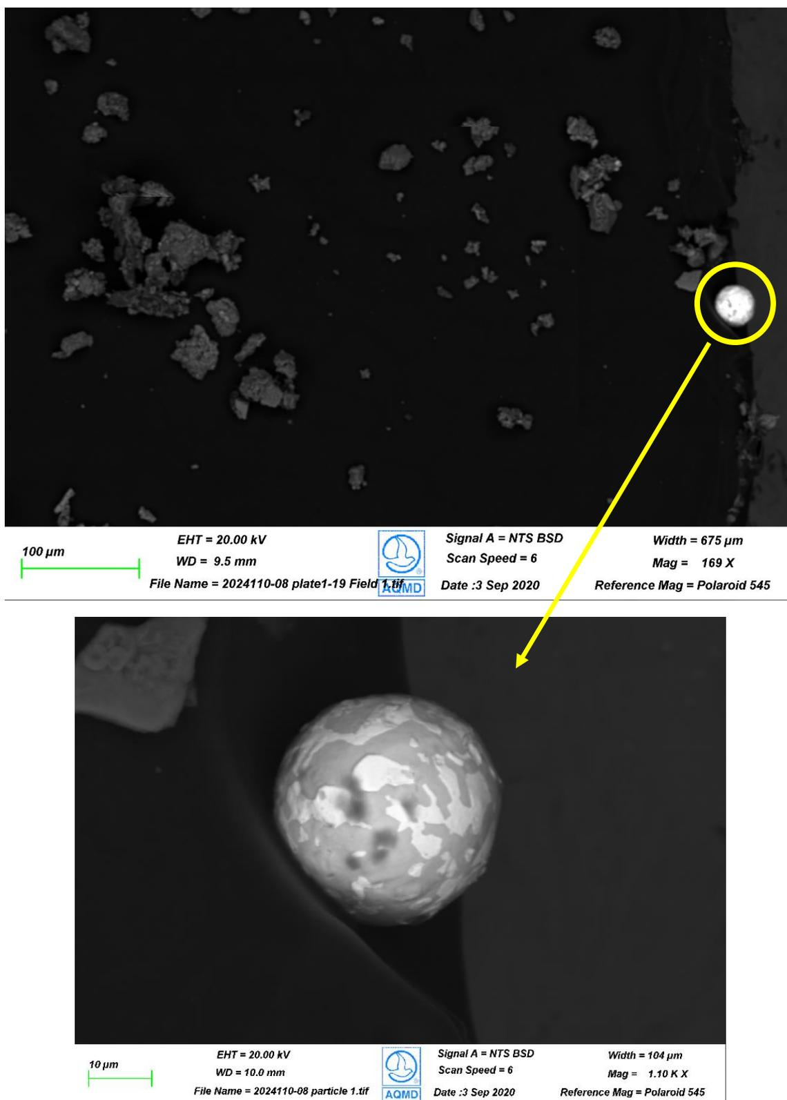
**Figure 3.** Westside #1: Spherical particle containing Pb and Sn. Composition, shape and surface texture resemble particle formed from a hot process such as soldering/welding.
