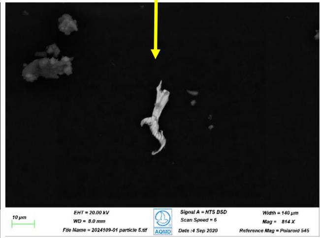
**Figure 2.** Southeast Middle School: Two metallic particles containing Cr and other metals. Composition, shape and surface texture resemble particle from metal grinding or shaving.
