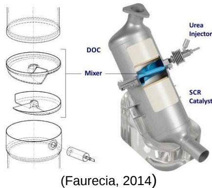
Figure III-5: SCR BlueBox Compact Mixer
