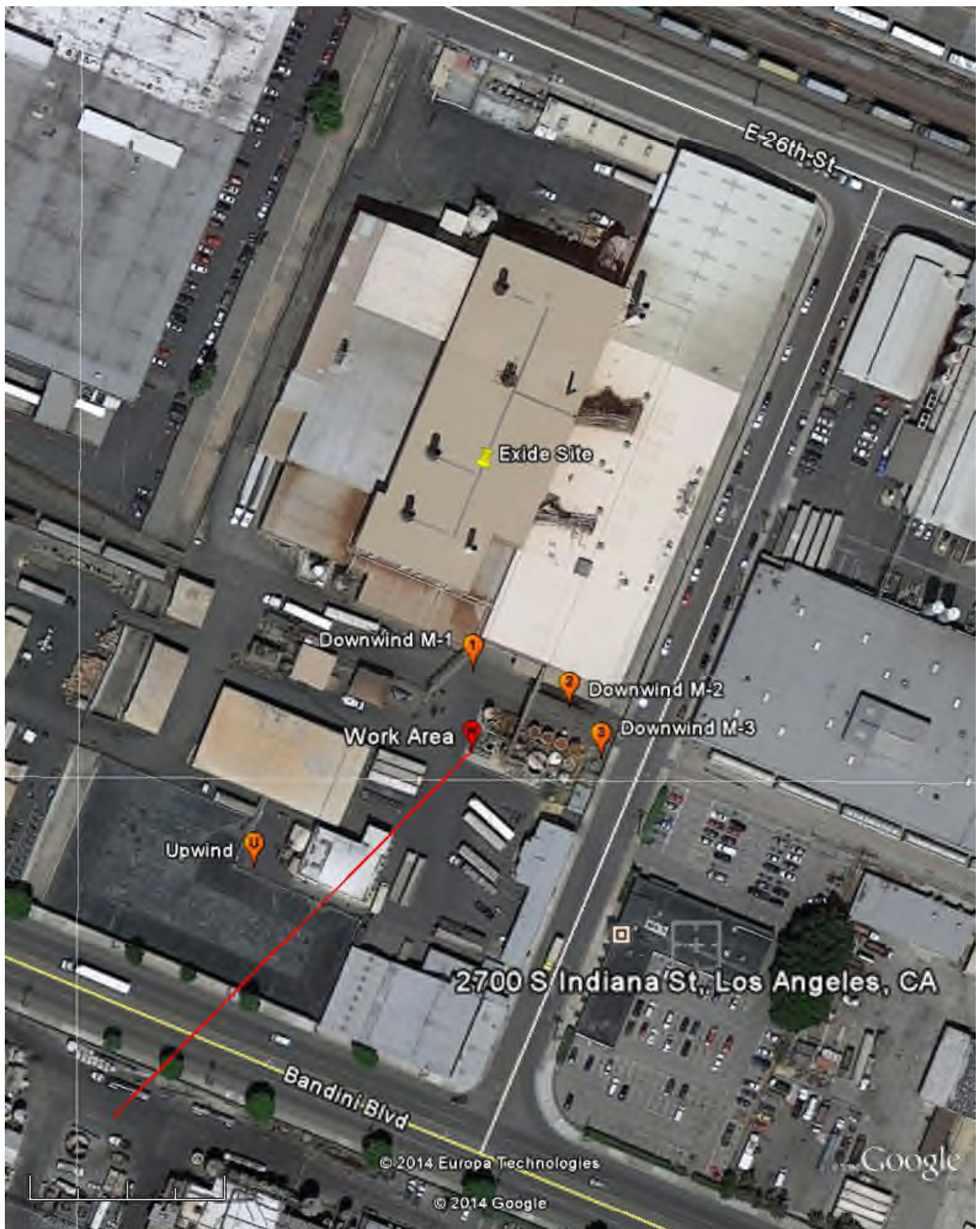
EX 35 SAND FILTER TANK REPAIRS DUST TRAK MONITORING LOCATIONS
