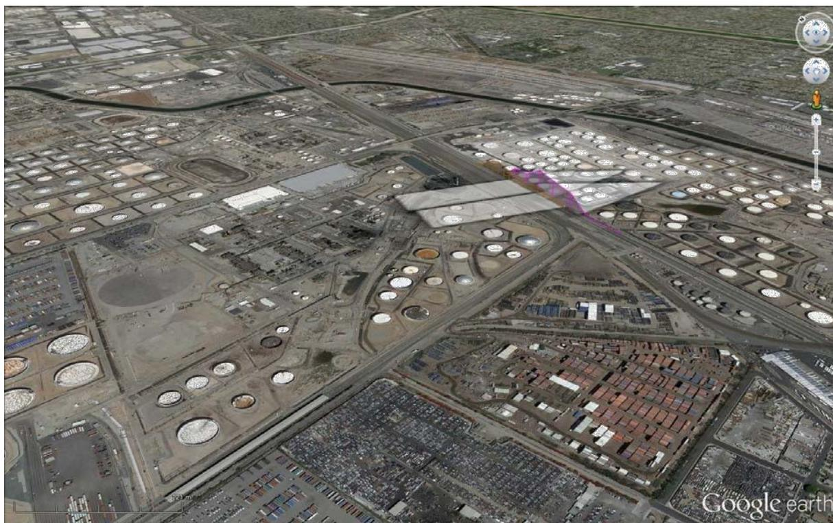
Figure 17 DOAS measurements taken at the Phillips refinery showing NO<sub>2</sub> (brown) and SO<sub>2</sub> (pink) emissions plumes (October 15, 16:10). North is to the upper left of the figure.
