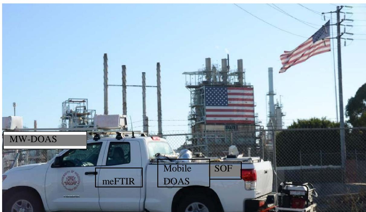
Figure 1. The measurement truck used these measurements.
