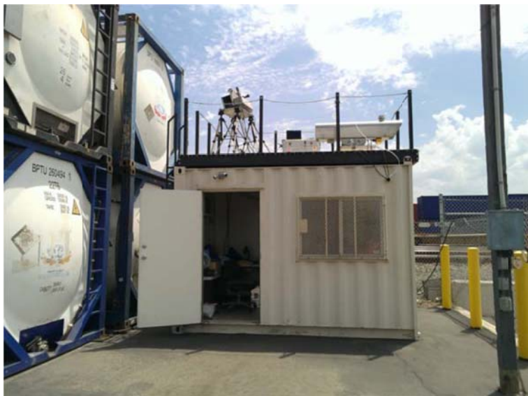
Figure 5.4: Photograph of the I-DOAS instrument on top of the container at the AQMD monitoring site in Carson.
