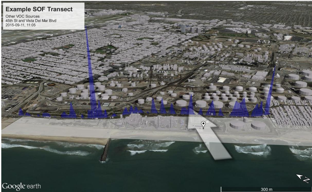
Figure 23. Example of a SOF measurements of a VOC source west of Vista Del Mar Blvd in Long Beach, 11 September 2015, 11:05. Alkane column is shown as a blue curve with apparent height proportional to gas column (10 m equivalent to 1 mg/m<sup>2</sup>, max 30 mg/m<sup>2</sup>). Wind direction during the measurement is indicated by the white arrow, measured with the FluxSense 10m wind mast. Map from Google Earth™ 2016.
