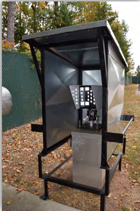
Figure 8. An example of a UVDOAS retroreflector (may not be configuration of actual installation).
