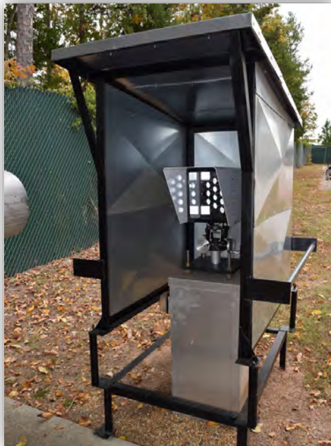
Figure 17. An example of a UV-DOAS retroreflector (may not be configuration of actual installation).
