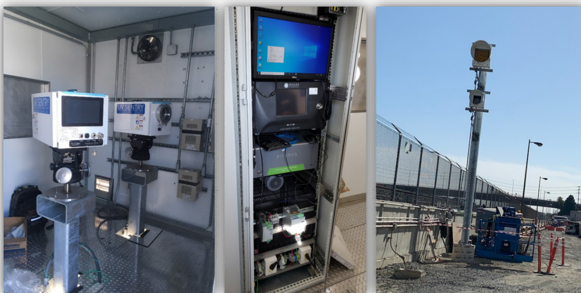
Figure 8. An example of two UV-DOAS analyzers, the point-monitor rack inside the communications cabinet, and a retroreflector tower with both a UV-DOAS and FTIR retroreflectors,
