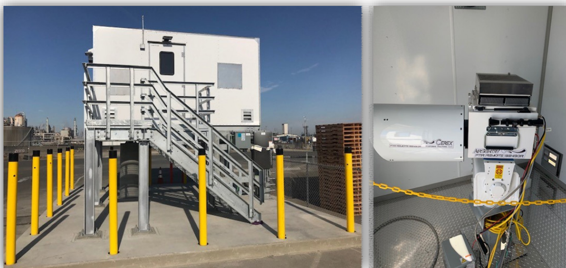
Figure 7. An example of an analyzer shelter (left) and an FTIR system (right).
