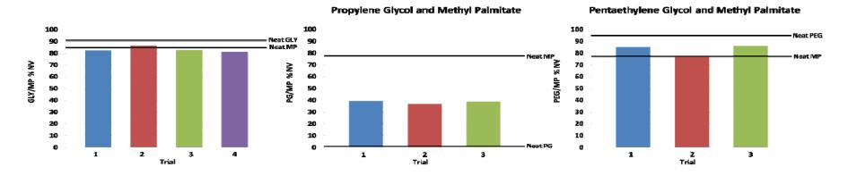
MP and test compounds not miscible Variable GC FID area ratios Variable %NVs (above)
