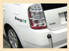
pioneered the engineering and development of the plug-in hybrid-electric vehicle Toyota Prius retrofit. This modified vehicle is designed to achieve more than 100 mpg for the first 50 to 60 miles of a user's daily commute.
