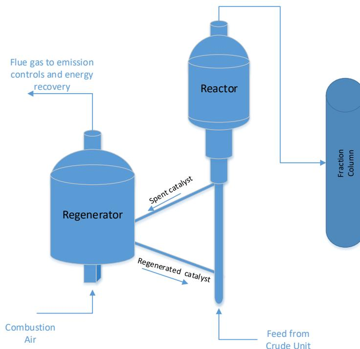
**Figure D-1. Simplified Schematic of FCCU Process**
