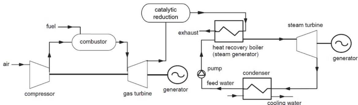
**Figure E-1. Combined Cycle Gas Turbine Diagram**
