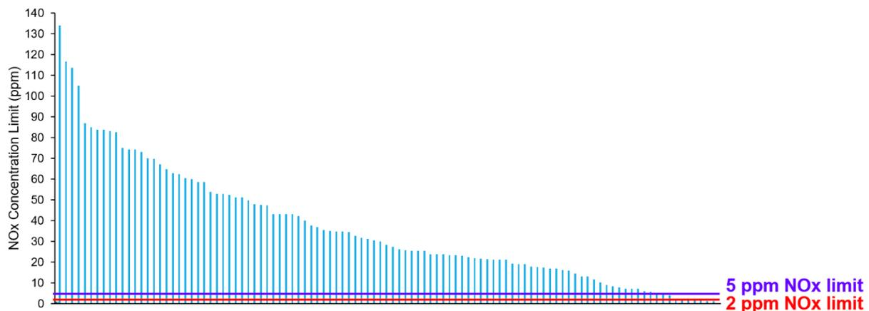
**Figure 1-2. NO<sub>x</sub> Concentration Levels of Boilers and Heaters  $\geq$ 40 MM Btu/hr**
