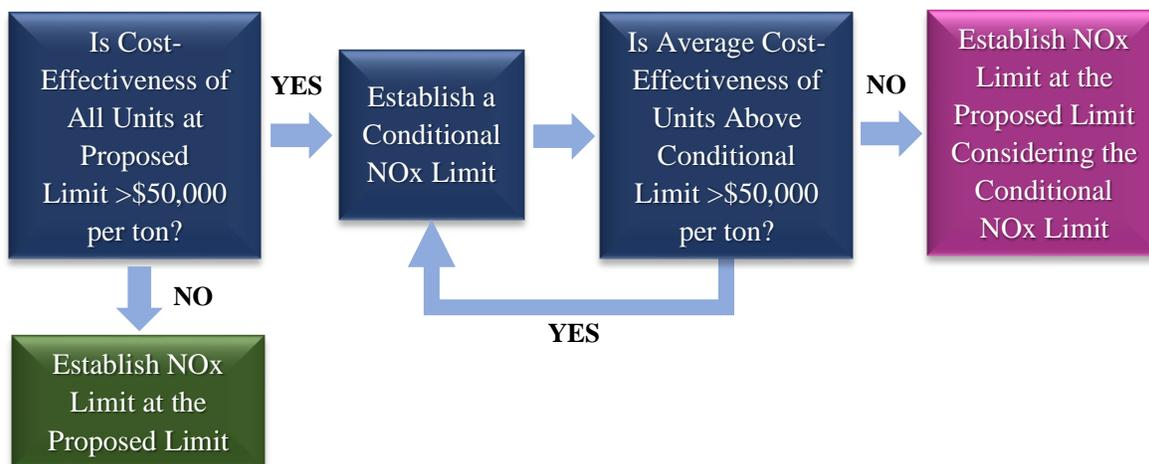
**Figure 2-6: Process to Establish Conditional NOx Limits For Large Process Heaters**
