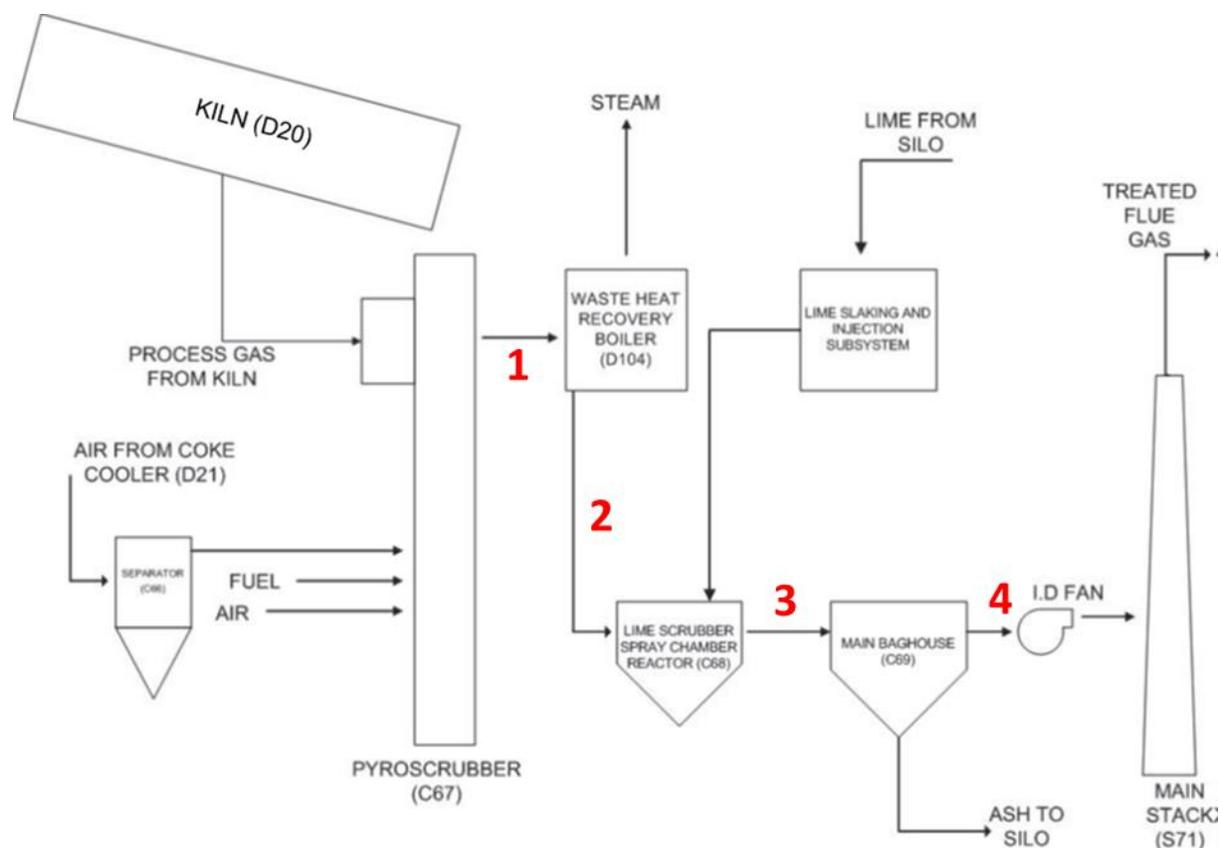
**Figure C-1. Coke Calciner Process and Potential Locations for NO<sub>x</sub> Control (Numbered in Red)**
