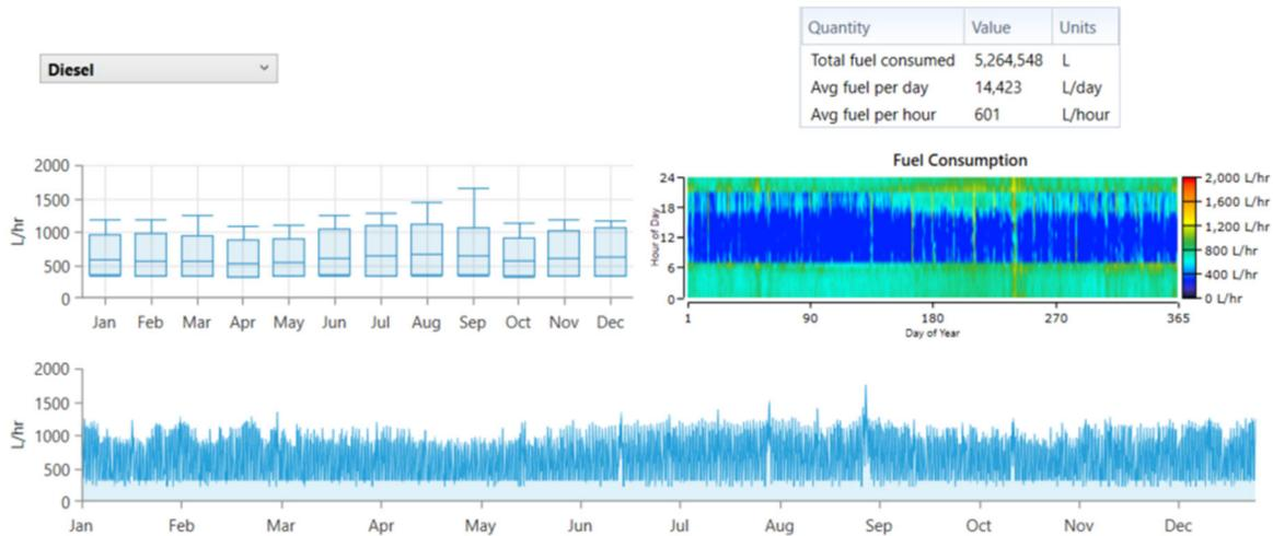
Figure 3: Diesel fuel consumption for Configuration 2
