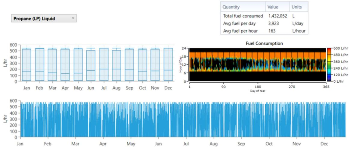
Figure 2: Propane fuel consumption for Configuration 2
