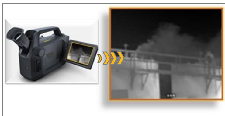
Figure 2.4 – OGI Camera Imaging
