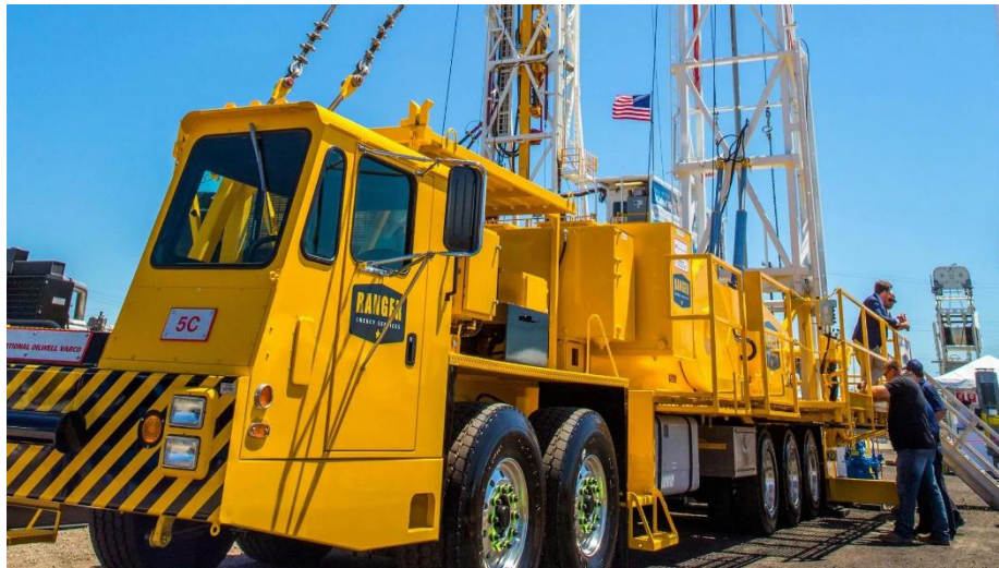
Figure 2: A Workover Rig Used in the Oil Production Field
