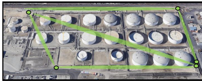
Figure 4.10 – Implementation of Open Path Detection (Example)
