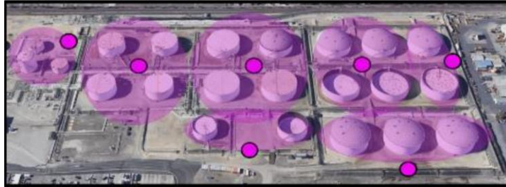
Figure 4.11 – Implementation of Fixed OGI Devices (Example)
