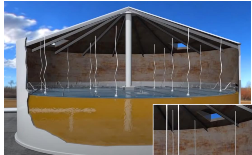
Floating roof with cable suspension system
