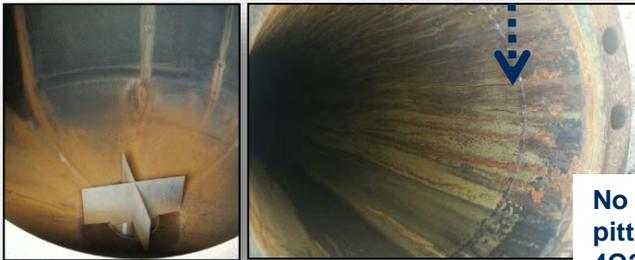
No signs of corrosion, damage, pitting or H2 grooving during the 4Q2014 inspection of 1<sup>st</sup> CDAlky unit and 3Q2017 inspection of 2<sup>nd</sup> unit
