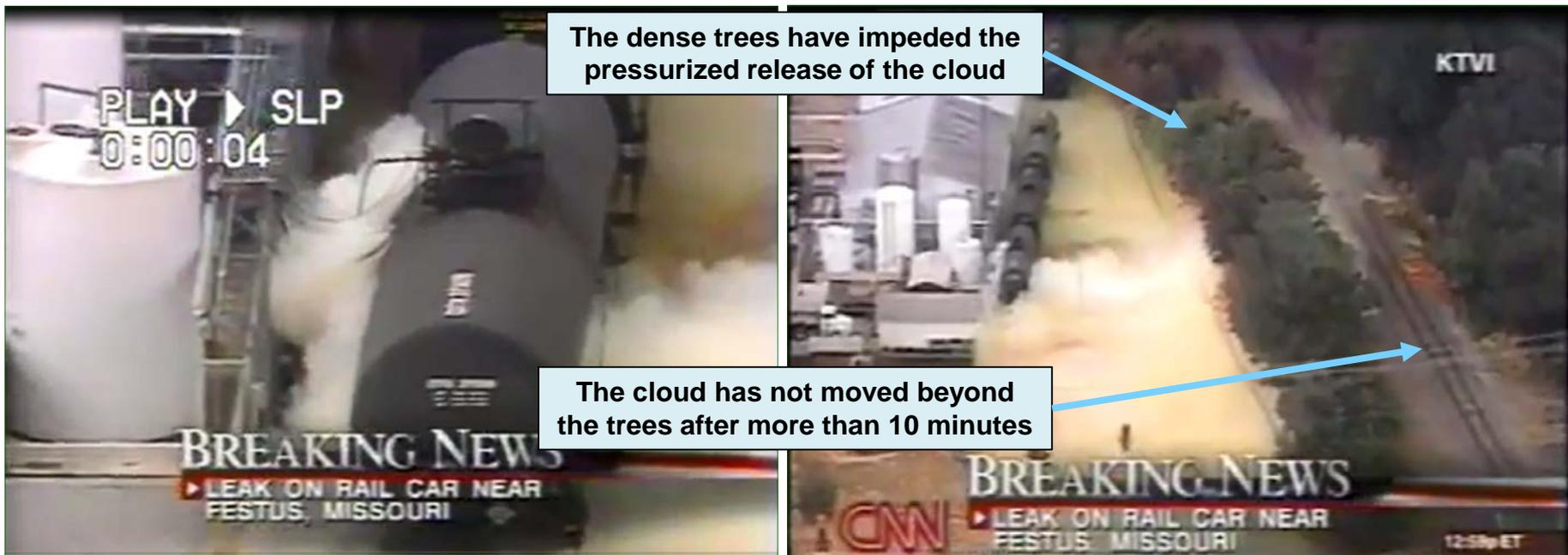
**A Chlorine Leak from a Railcar Demonstrates the Effect Physical Structures Have on a Toxic Cloud's Speed of Travel**
