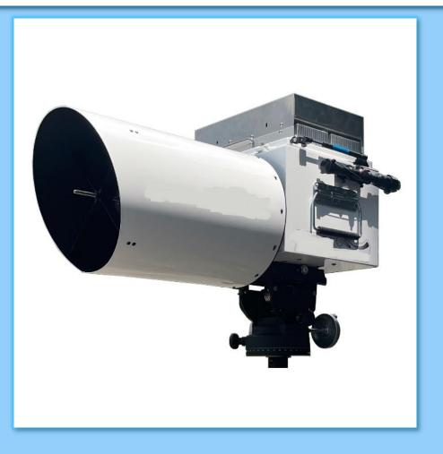
Open Path devices produce a beam across an area and quantify targeted emissions including VOC across path
