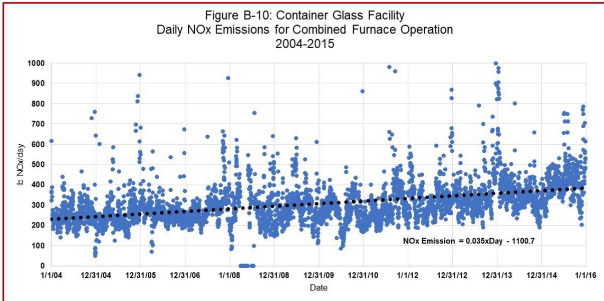
Figure B-10, NO<sub>x</sub> is seen to have increased approximately 0.035 lbs of NO<sub>x</sub> per day over a twelve year period. Since this represents two furnaces in operation, the corresponding NO<sub>x</sub> emissions increase per furnace would be approximately 0.0175 lbs of NO<sub>x</sub> per day or 6.4 lbs per year per furnace. The expected NO<sub>x</sub> increase due to the aging experienced by a furnace may be approximately 96 lbs over a 15 year operational cycle.
