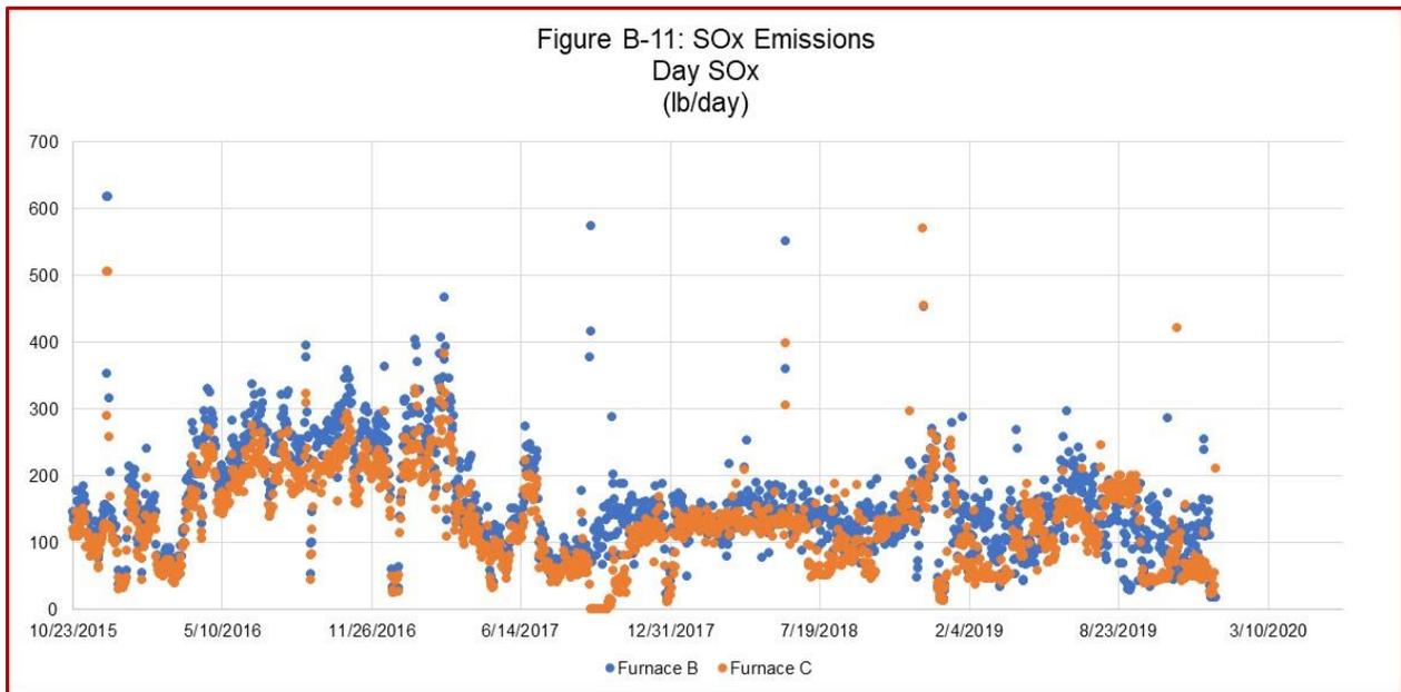
Figure B-12 illustrates the SOx emissions per day based on the ratio of emissions to glass pulled from the container glass melting furnaces from CY 2016 to CY 2019.
