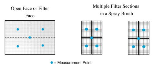
For an enclosed spray booth, the inward face air velocity measurements shall be taken between 6 and 12 inches from the exhaust filters.
