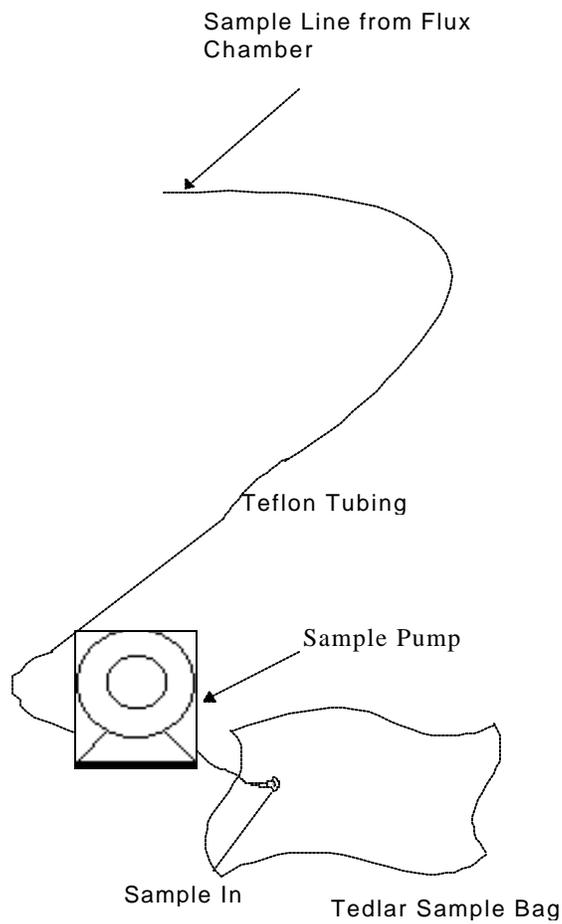
**Figure 4 Integrated Gas Sampling Apparatus**
