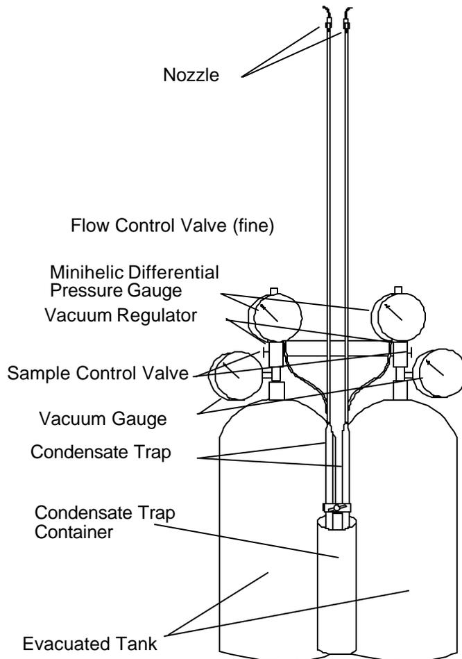
**Figure 6 Method 25.1 Sampling Apparatus**
