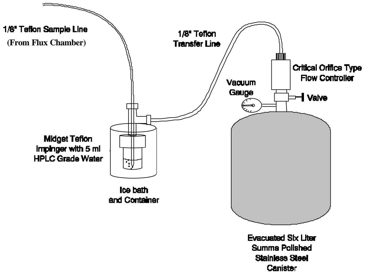
**Figure 5 Modified 25.1 Sampling Apparatus**
