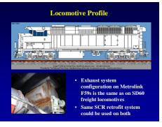
the exhaust to achieve this level. More compact SCR systems being developed in Europe for use on trucks could be applicable to locomotives here, and possibly to harbor craft. Tests on marine engines indicate that the systems reduce not only NOx but also PM, functioning as a DOC and burning the organic component of the PM.
