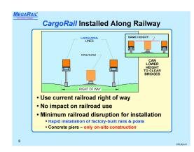
Low-noise heavy-duty rubber truck tires run on flat steel in this system. The trams can go up grades, in all weather types, and have no turning limitations. The propulsion system is in each tram unit wheel: permanent magnet hub motors such as are used in some electric buses. Power is delivered via side rails that are enclosed to ensure safety. The overhead structure has an open design so as not to block light beneath it. The company has built and tested
