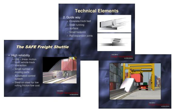
The vehicles have aerodynamic front and back ends (they are bi-directional) and would move about 35-40 miles per hour. The guideway is laid on a concrete base and is not envisioned as an elevated structure in this system. Communications run to and from the vehicles through the energy source on the guideway. The specifics of terminal design would be determined based on desired use – no general layout has been determined.
