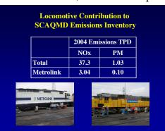
emissions since locomotives often idle during this time. Line haul locomotives can spend 40% of their time idling and switchers as much as 90%. The two-stroke engines used in many diesel locomotives produce substantial emissions from lubricating oil.
