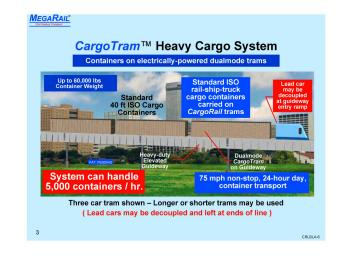
The line-haul (guideway) operation is fully electrified and would not generate any emissions at the source. Off the guideway at terminals, the tram is a hybrid that would be fueled by compressed natural gas (CNG). The guideway is steel rather than concrete, and is bolted together on site. The only site construction is concrete support piers; all other components are factory-built and brought to the site.
