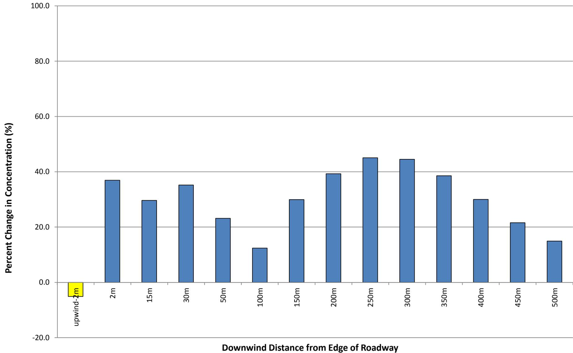
**Figure 2 - Soundwall - 500 feet long, 5 meters high, configuration 1**
