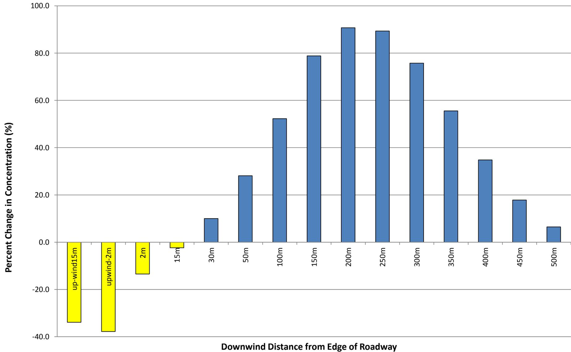
**Figure 8 - Soundwall with Fans - 50% fan intake, 3.3 meters apart**
