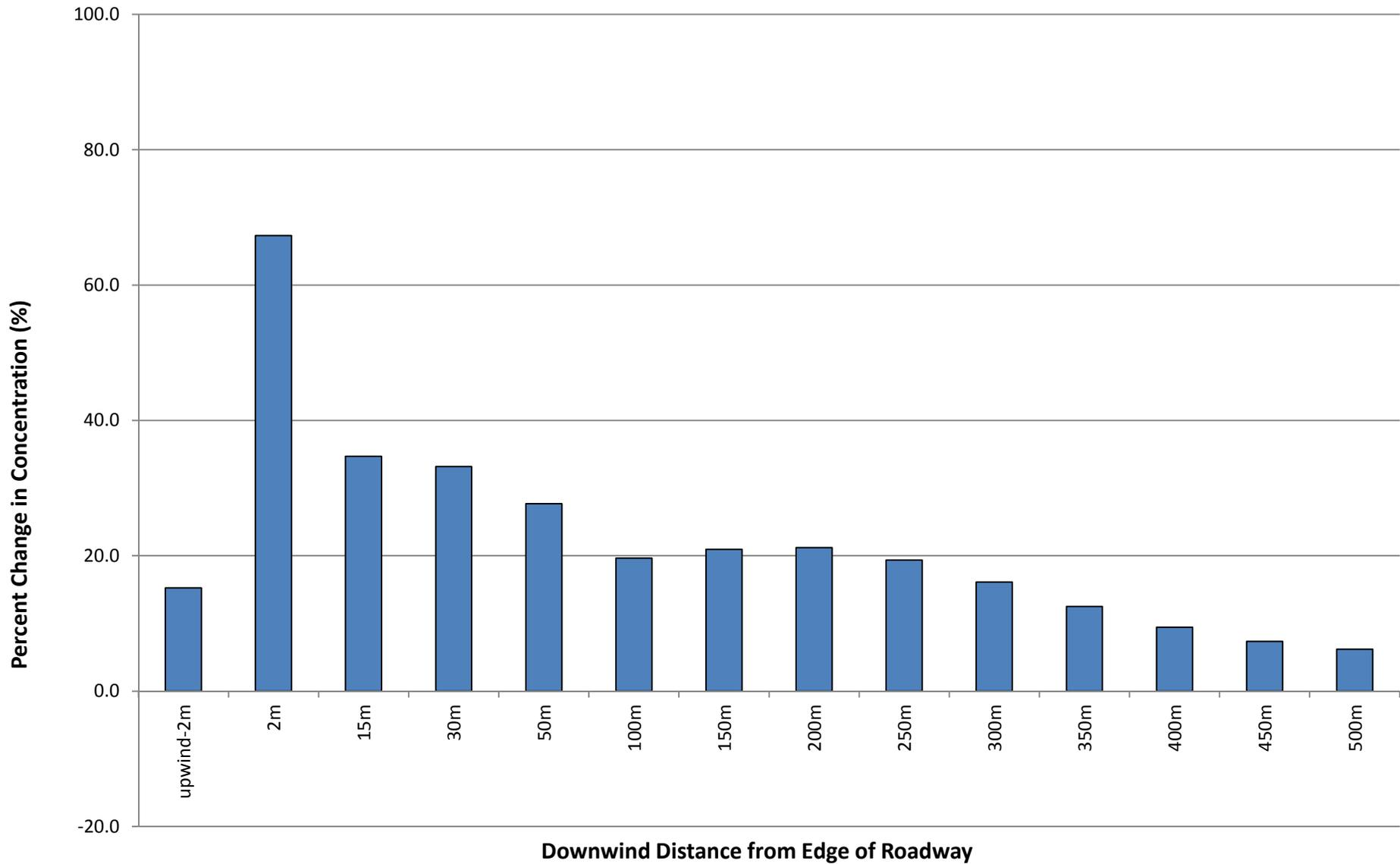
**Figure 3 - Soundwall - 500 feet long, 5 meters high, configuration 2**
