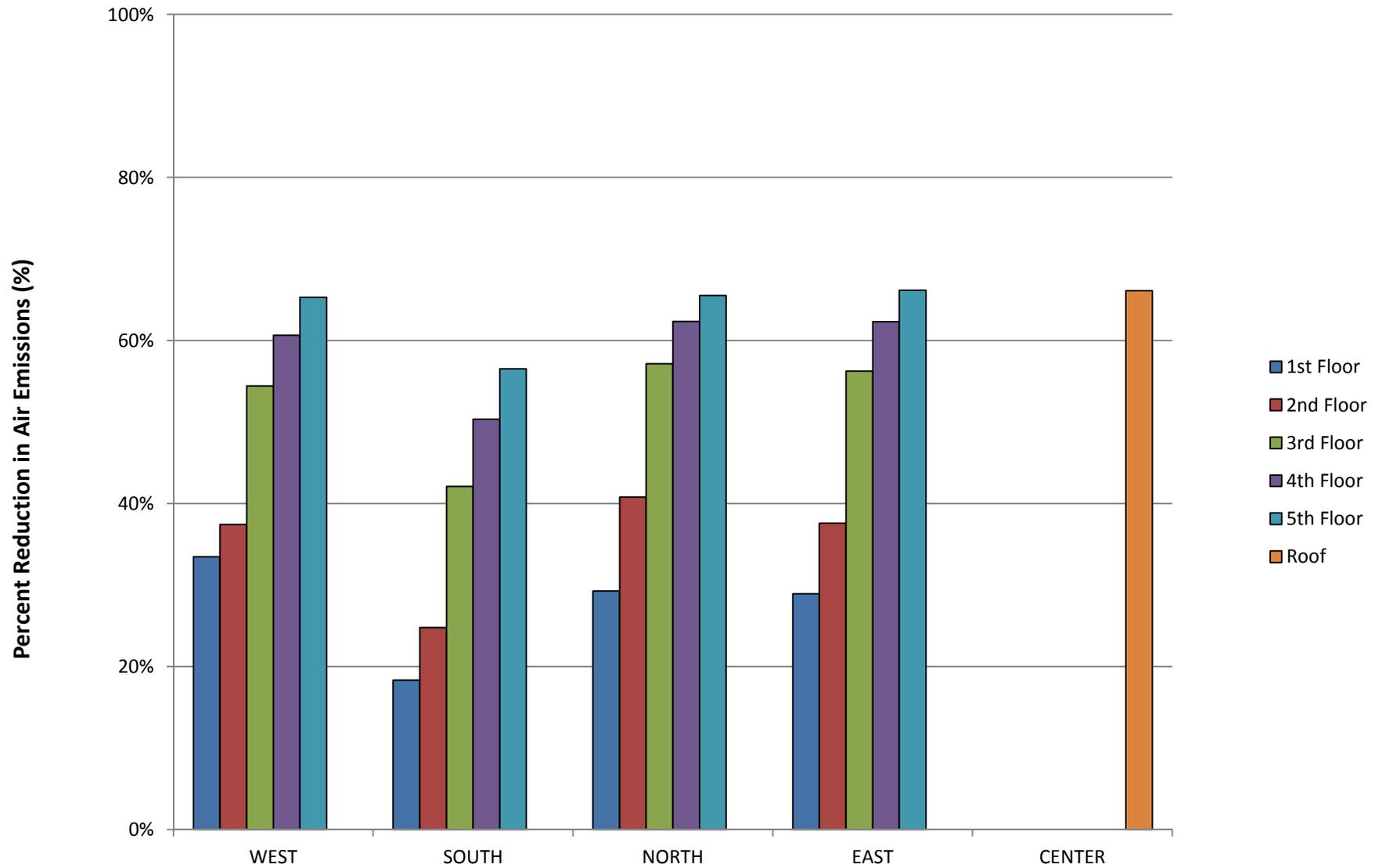
**Figure 19 - 3-Story Building, with Soundwalls - 5 meter high,
