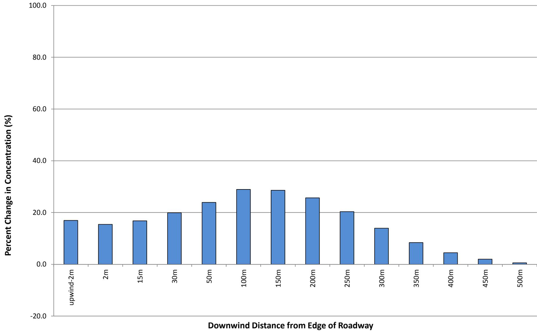
**Figure 7 - Soundwall with Fans - 75% fan intake, 3.3 meters apart**
