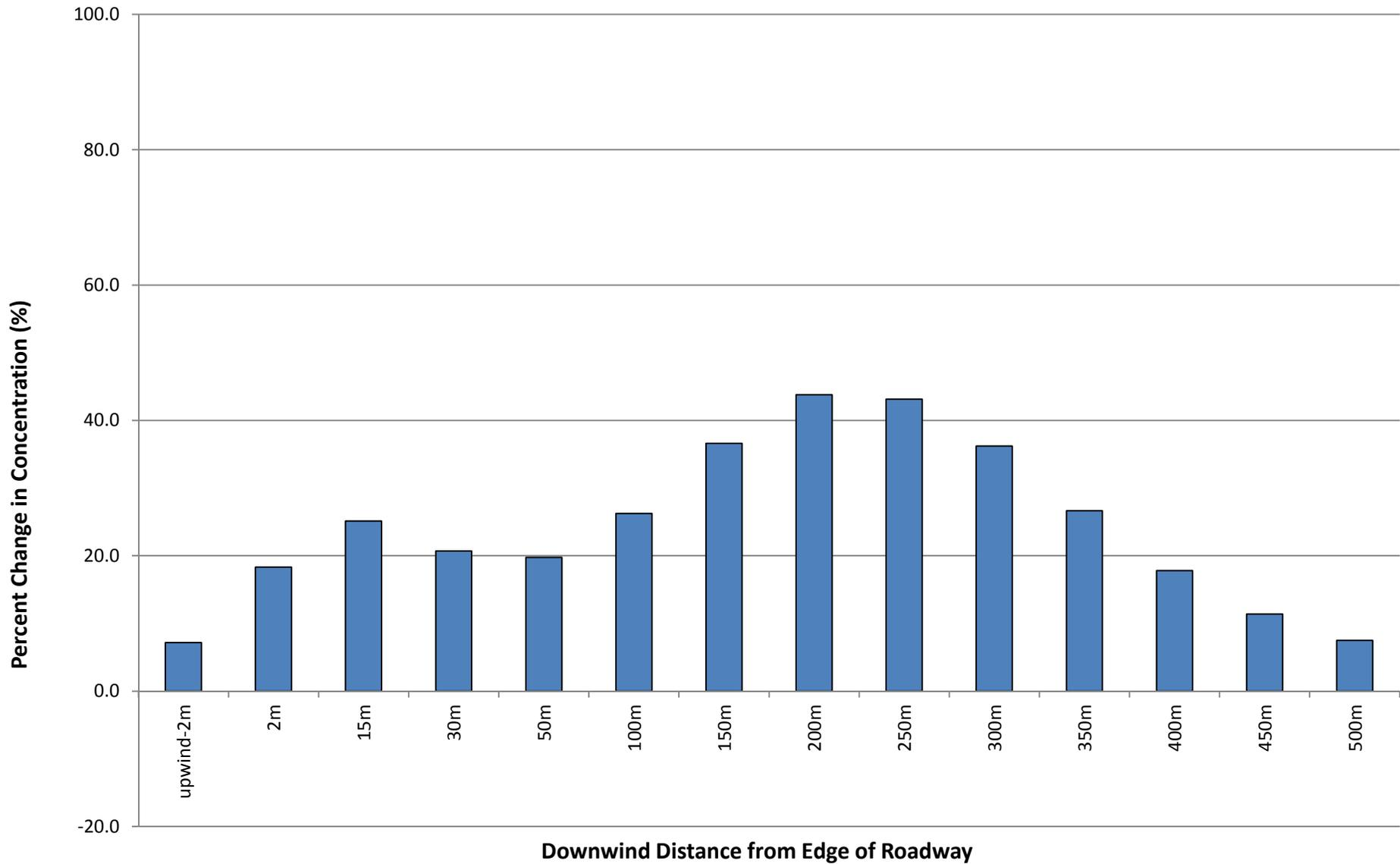
**Figure 4 - Soundwall - 1,000 feet long, 5 meters high, with 100 foot gaps**
