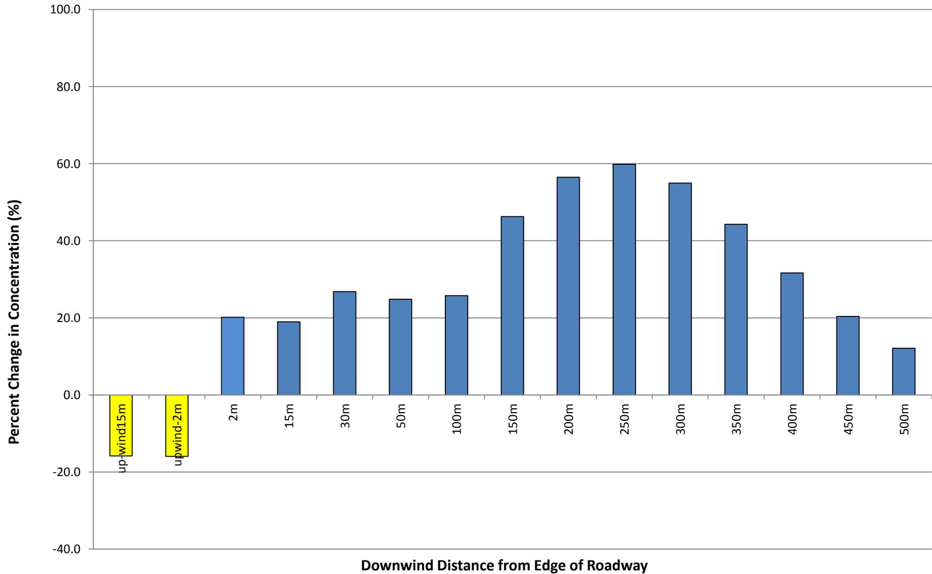
**Figure 10 - Soundwall with Fans - 75% fan intake, 15 meters apart**
