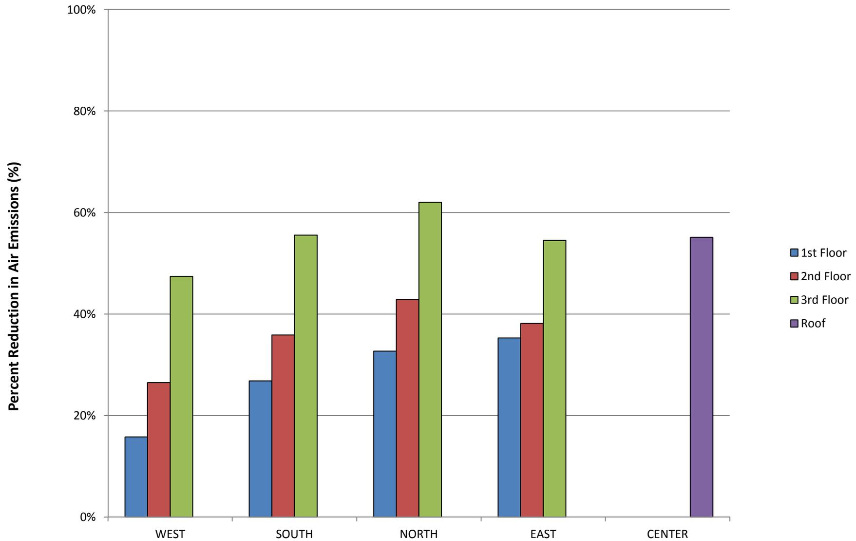
**Figure 14 - 3-Story Building, with Soundwalls - 5 meter high,
