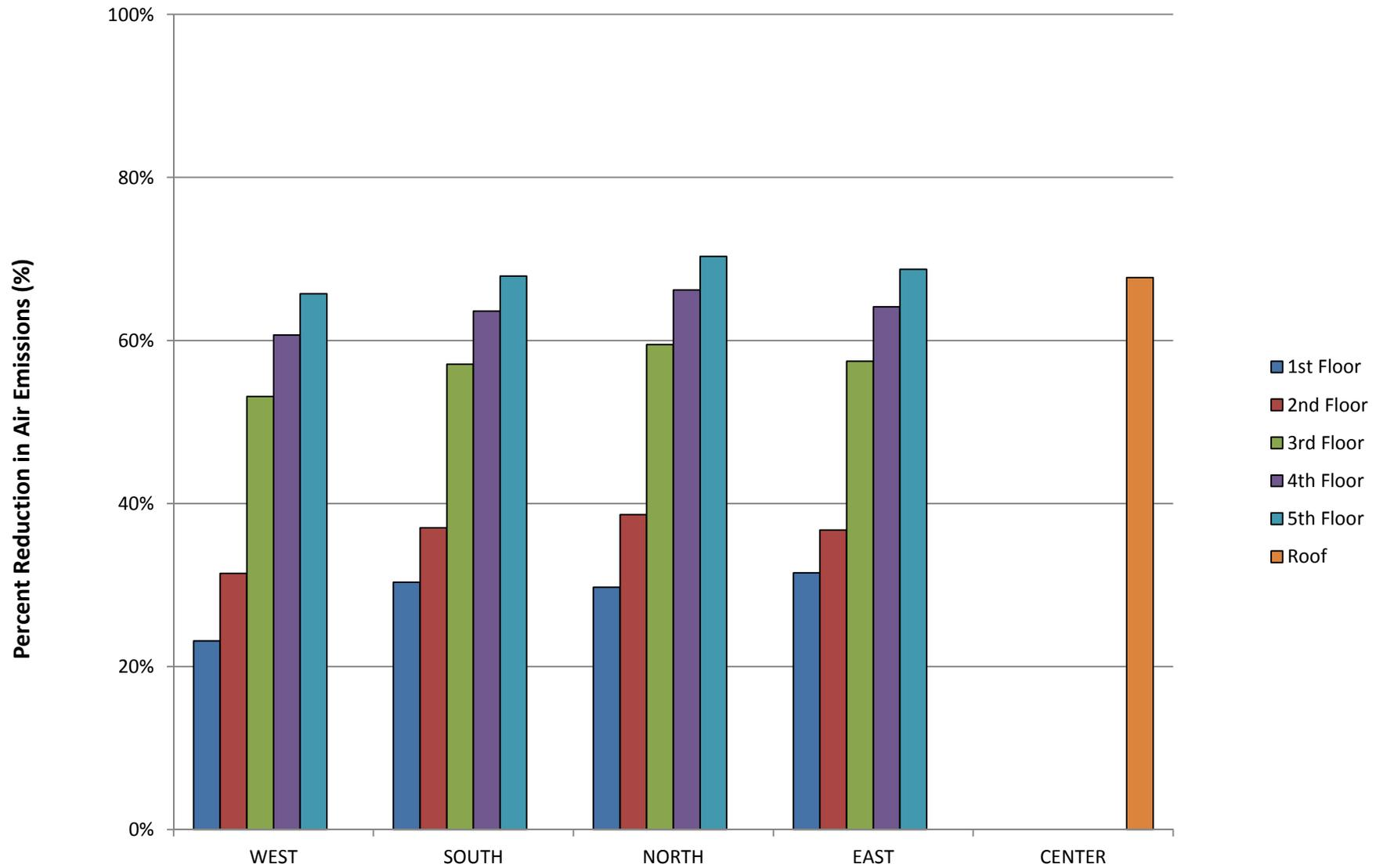
**Figure 16 - 5-Story Building, with Soundwalls - 5 meter high,
