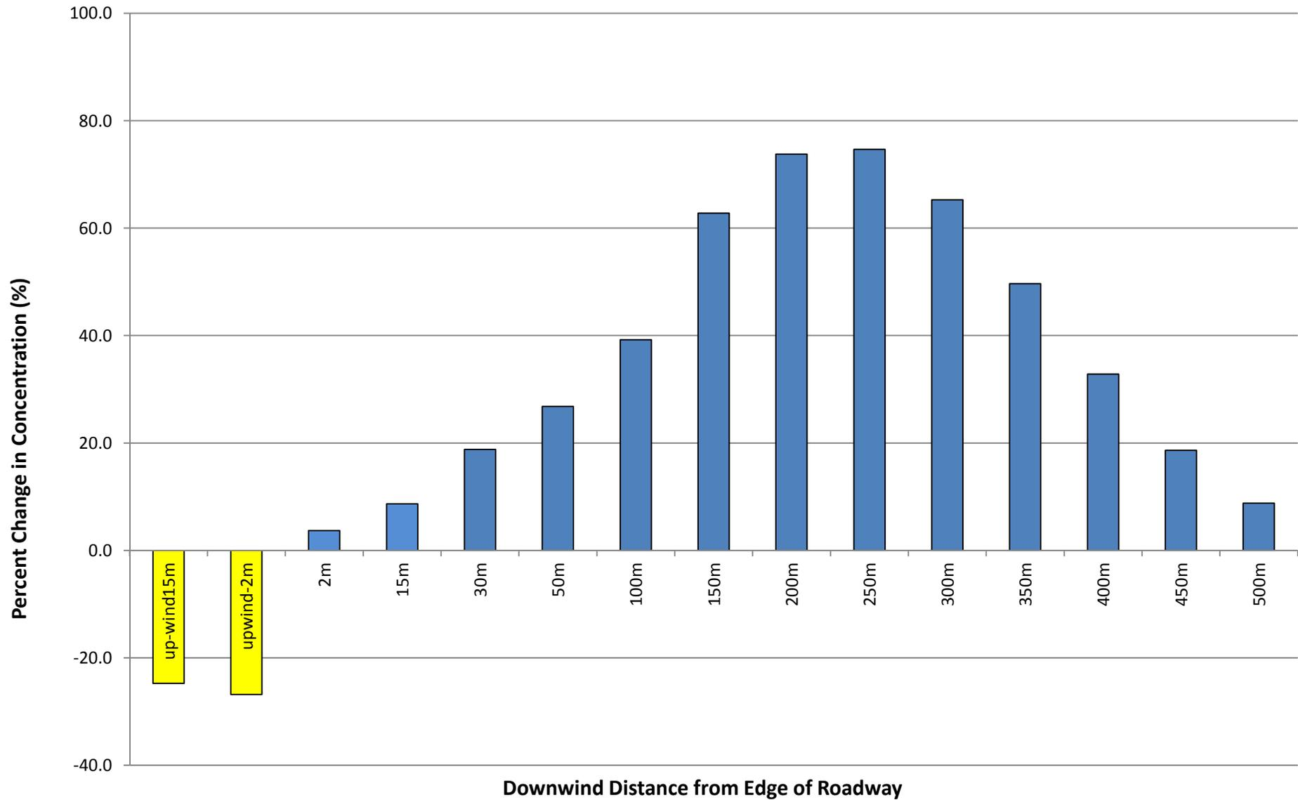
**Figure 12 - Soundwall with Fans - 25% fan intake, 15 meters apart**
