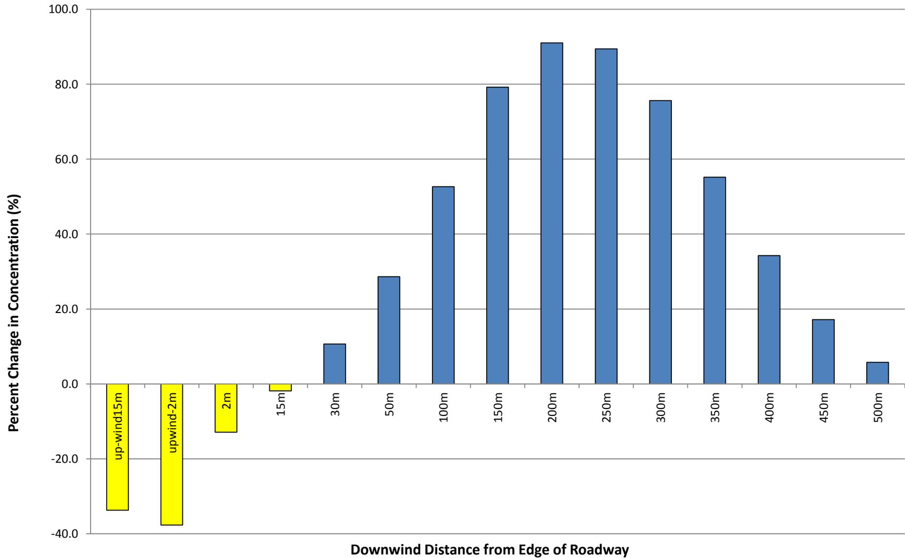
**Figure 11 - Soundwall with Fans - 50% fan intake, 15 meters apart**
