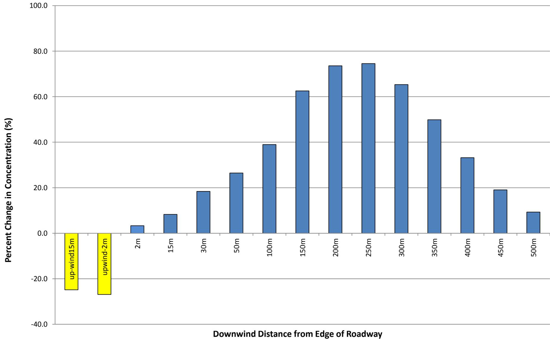
**Figure 9 - Soundwall with Fans - 25% fan intake, 3.3 meters apart**
